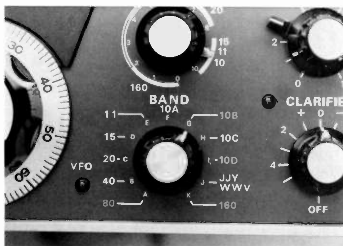
Photo A. The WWV position on the bandswitch is used to cover 10.0 to 10.5 MHz, which includes the 30-meter band. The 11-meter position on the bandswitch can easily be modified to cover 24.0 to 24.5 MHz, which includes the 13-meter band, at a later date. Likewise, the 160-meter position could be sacrificed to cover 18.0 to 18.5 MHz, which includes the 17-meter band.
