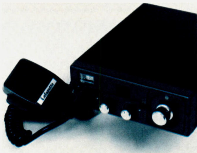
Front view of converted Lafayette rig. The CB channel switch has been replaced with a 10-position rotary. A pair of 7-segment LEDs have been added for direct frequency read-out. Three toggle switches provide display on/off, simplex/repeat, and add 10-kHz to operating frequency.
