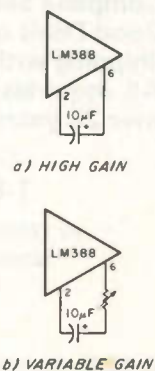
Fig. 8. LM388 gain control.
