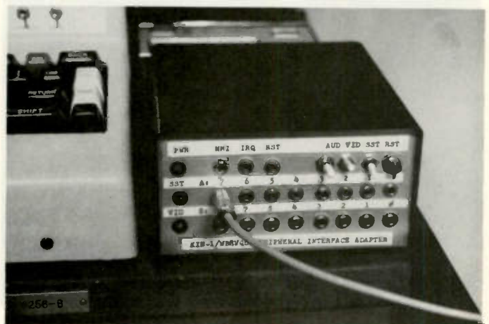
Close-up of home brew interface box. Others might consider bringing all peripheral pins out to miniature phone jacks and all controls to outboard switches.
