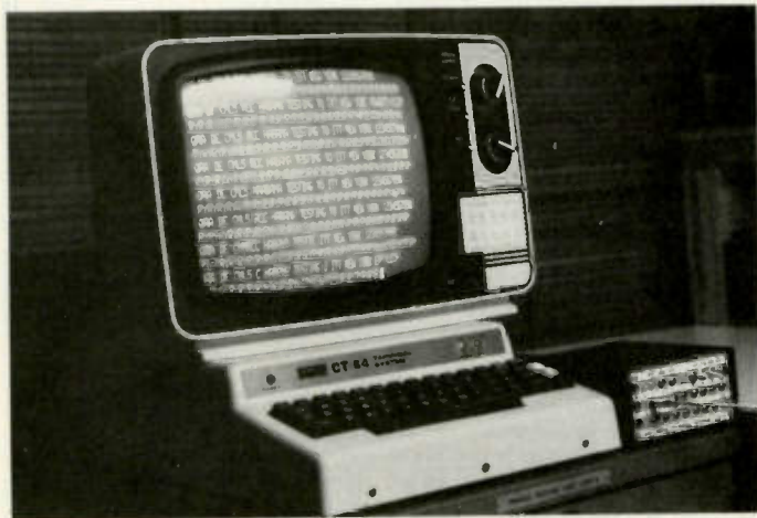
Computer-generated RTTY station: Note use of inexpensive black and white portable TV, SWTPC CT-64 video terminal, and home brew interfacing box.
