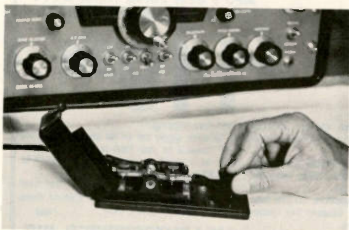
Here is a German Baumuster T1 military key of the 1930s. "This is my favorite hand key because the adjustments are precise and the concave knob gives it a good feel," says John Elwood, who purchased the key from Louise Moreau W3WRE. In the background is John's Hallicrafters SX-101A receiver. That's John's precise fist in action.
