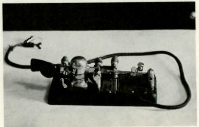
This Horace G. Martin Rotoplex key built for the US Army Signal Corps during World War II has a black crackle finish on a steel base and is mounted on a quarter-inch rubber mat.
