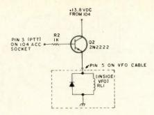
Fig. 5. Vfo relay switching circuit.
