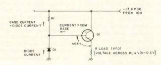
Fig. 4. Power supply simplified circuit.
