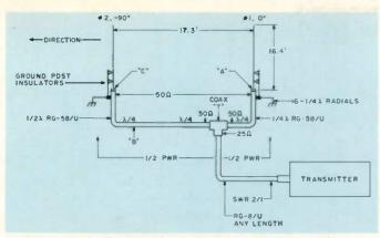
Fig. 1. Method of feed for the 2-element phased array.
