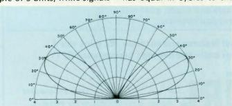
Fig. 9. Vertical angle of radiation of a half-wave dipole at a height of 1/2-wave above a perfectly conducting ground.
