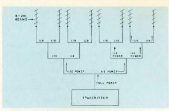
Fig. 4. Feeding eight 2 meter beams in phase with equal power. Feedlines to all beams are of equal length for inphase operation. This is the type of phasing harness to use for broadside directivity of the 8-element array.
