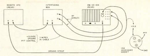
Fig. 2. Interfacing cable layout.
