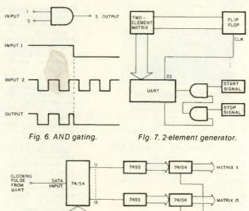
Fig. 8. Banking matrix using a 74154.
