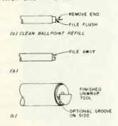
Fig. 2. Unwrap tool construction.
