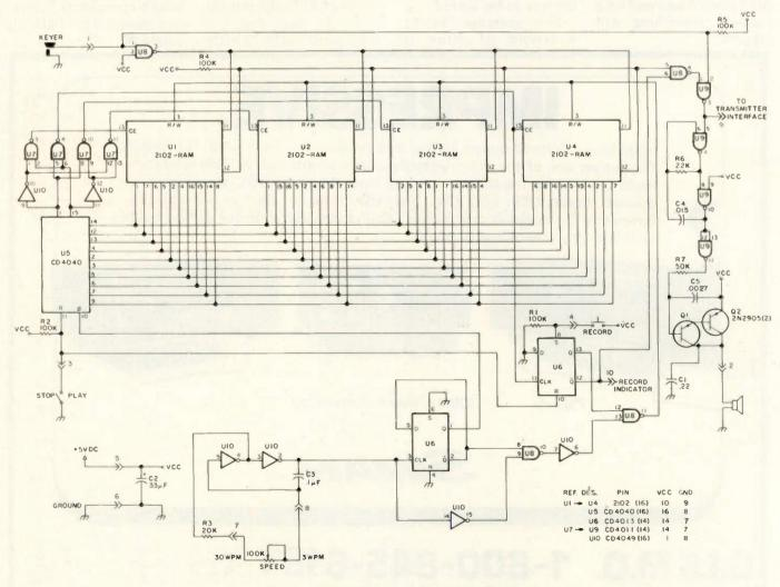
Fig. 1. Code Memory schematic diagram.
