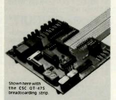
The FTK 6100 Universal Designer is an Indispensable aid to breadboarding digital IC's. It plugs directly into breadboards such as the Continental Specialties QT-47S, and provides the most often used inputs and outputs for circuit design.
