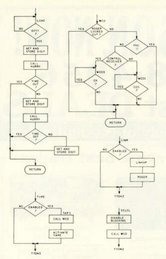
Fig. 4. Load, wait for carrier drop, link, tape, and selective call routines.
