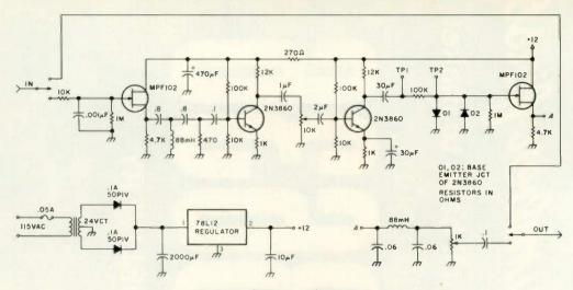
Fig. 2. Audio filter/clipper/filter.
