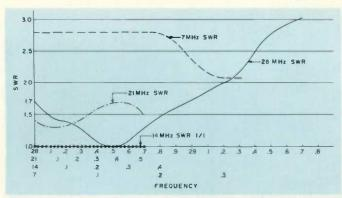
Fig. 11. Swr curves for 7 MHz through 28 MHz for the array.
