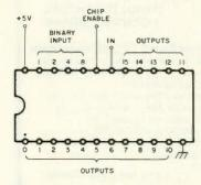
Fig. 2, 74154 data distributor pinout.
