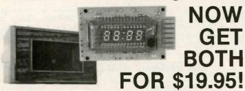
The MA1003 is a popular clock module that features blue-green fluorescent readouts (won't wash out in daylight), a highly accurate built-in timebase (excellent for mobile/portable operation and battery backup applications), and really easy assembly . . . add time setting switches, + 12V DC, and you're ready to go. So simple, it makes a great one evening project; so inexpensive, you can afford to have accurate, electronic time-keeping not only in your home but in your car, truck, or van.
