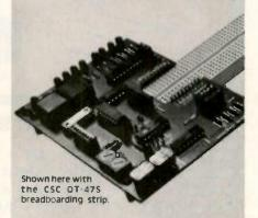
The FTK 6100 Universal Designer is an indispensable aid to breadboarding digital IC's. It plugs directly into breadboards such as the Continental Specialties QT-475, and provides the most often used inputs and outputs for circuit design.
