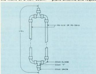
Fig. 5. 37.5-Ohm Q transformer—converts 25 Ohms to 56 Ohms.
