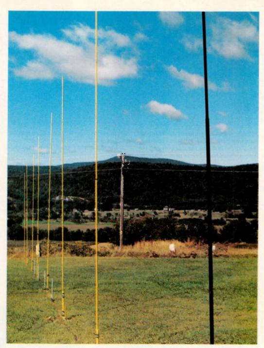
Looking west along the line of the array: The Connecticut River flows in the valley and the hills in the distance are in Vermont. Note that the top of the 7th element is just even with the horizon. A little trig with a pocket calculator tells us that our minimum angle of radiation is about 6 degrees.
