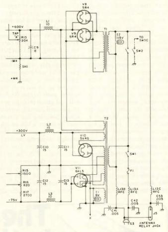
Fig. 1. Original Viking power supply diagram.
