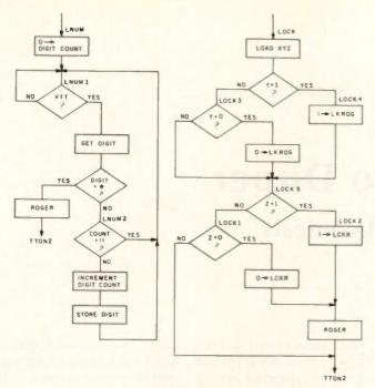
Fig. 10. Load number and lock routines.
