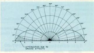
Fig. 10. Vertical angle of radiation from a half-wave vertical antenna whose center is 14-wave above a perfectly conducting ground.
