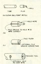
Fig. 1. Wire-wrap tool construction.
