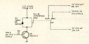
Fig. 6. Interface relay switching circuit.
