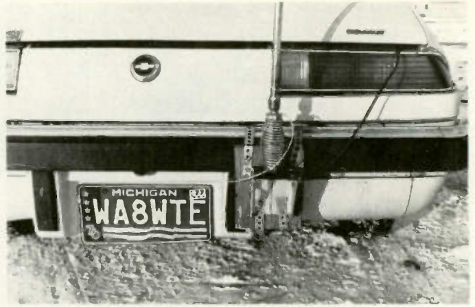
The $1.00 bumper mount attached to the Monza's rubber bumper. The coax braid must be securely grounded to the frame underneath.
