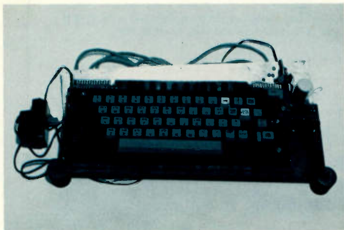
Photo A. Diode matrix (front) forms 8-bit binary code. The 13 ICs (back) provide logic to convert binary code to Morse code. Keying and VOX relays at lower right.
