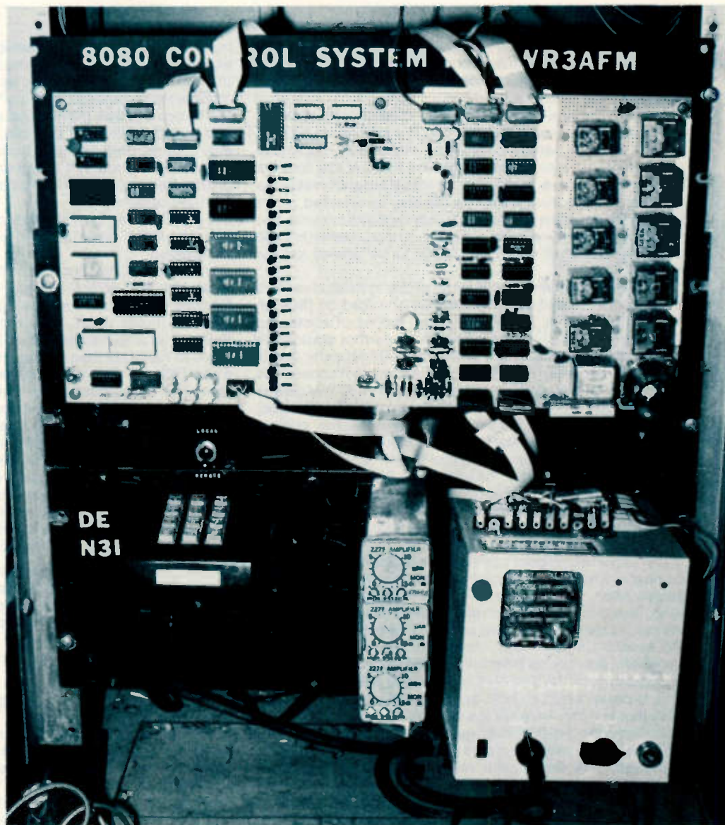
Control system connected to repeater.
