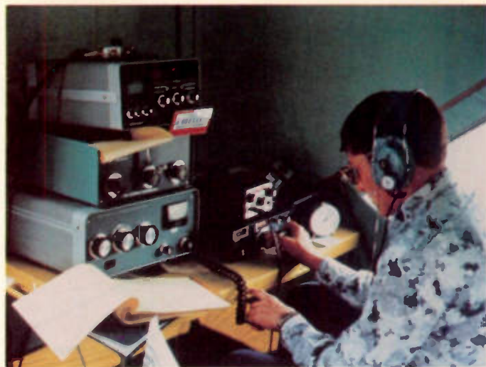
Doug DA2AJ in #2 operations tent. Audio processing gear, both TX and RX (VOMAX, AUTEC QF-1, respectively) proved to be quite effective during noisy and/or pileup conditions.
