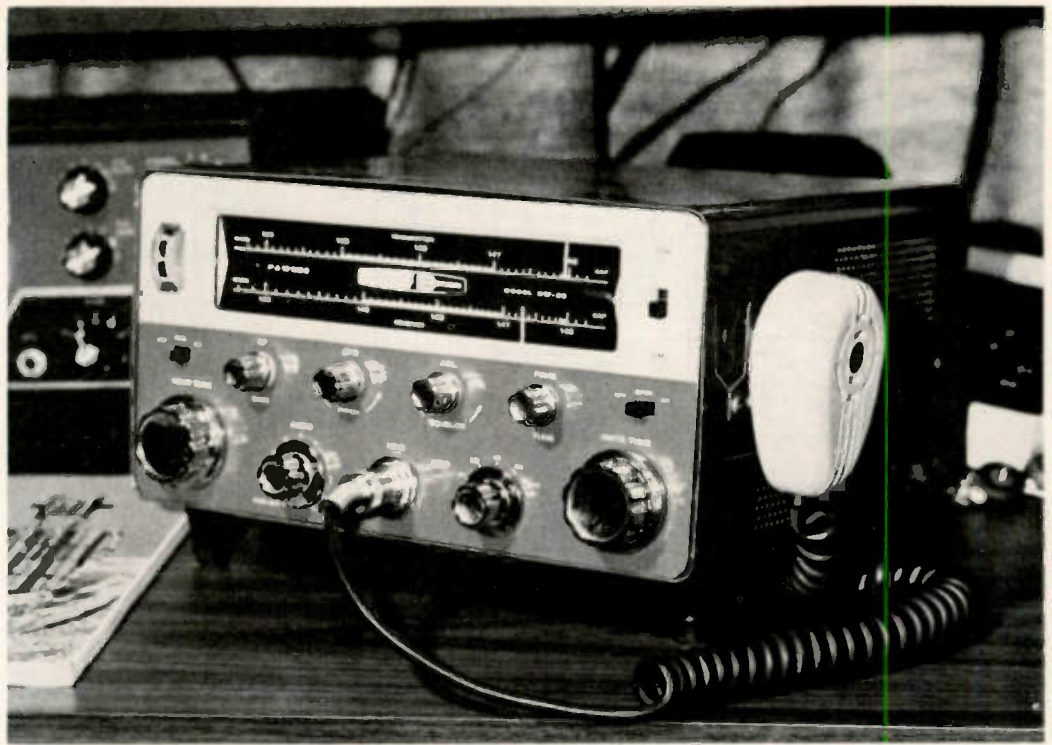
Heath's twenty-year-old two meter AM Pawnee transceiver is just too beautiful to become a museum piece. It's easy to recycle it for operation in the two meter FM band.
