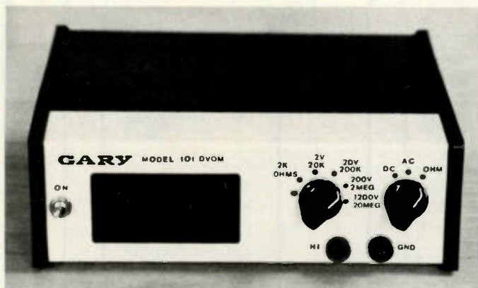
What would an article by Gary McClellan be without a Gary meter? This is the model 101 and it reads ac volts, dc volts, and Ohms.
