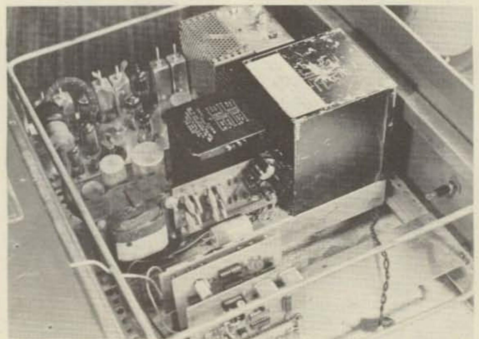
Photo D. Top view showing transmitter, power supply, and circuit boards. Note: AFSK board (outside) is a prototype.
