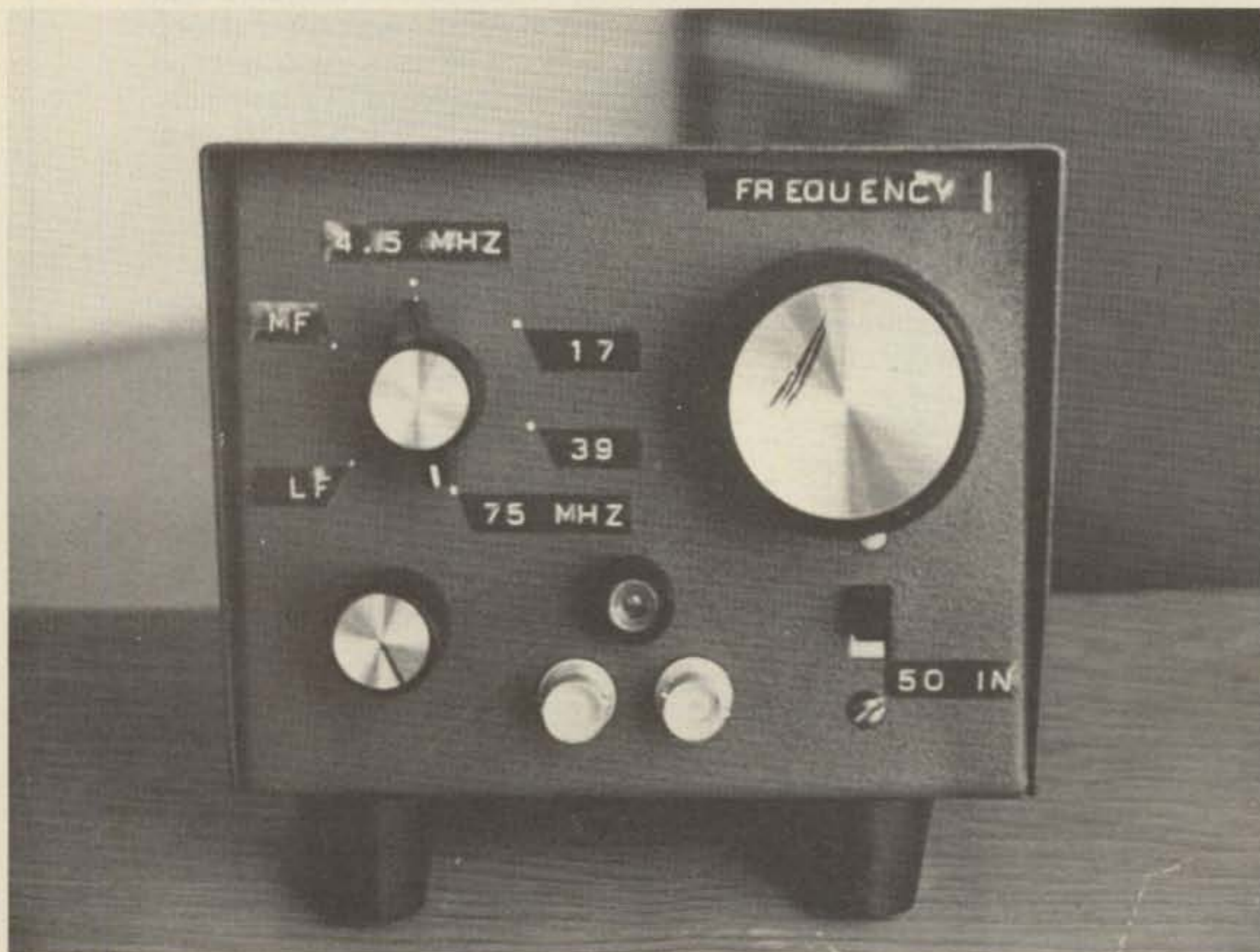
The rf signal generator has no frequency readout scale, for reasons explained in the text. Two BNC output connectors are used — one for the actual signal output, and one for connection to a counter.
