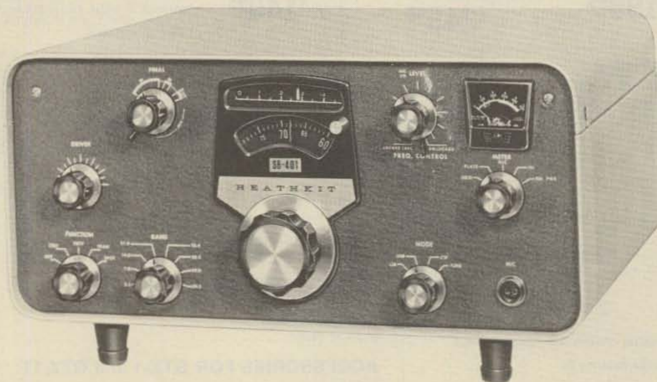
This popular amateur transmitter uses tubes all the way through, rather than solid state. Nonetheless, it serves as an excellent example of an SSB transmitter using the filter method to generate an SSB signal. Although presently superseded by solid state units, this model is still quite popular, and brings a good price at hamfests and in the want ads. (Photo courtesy of Heathkit.)
