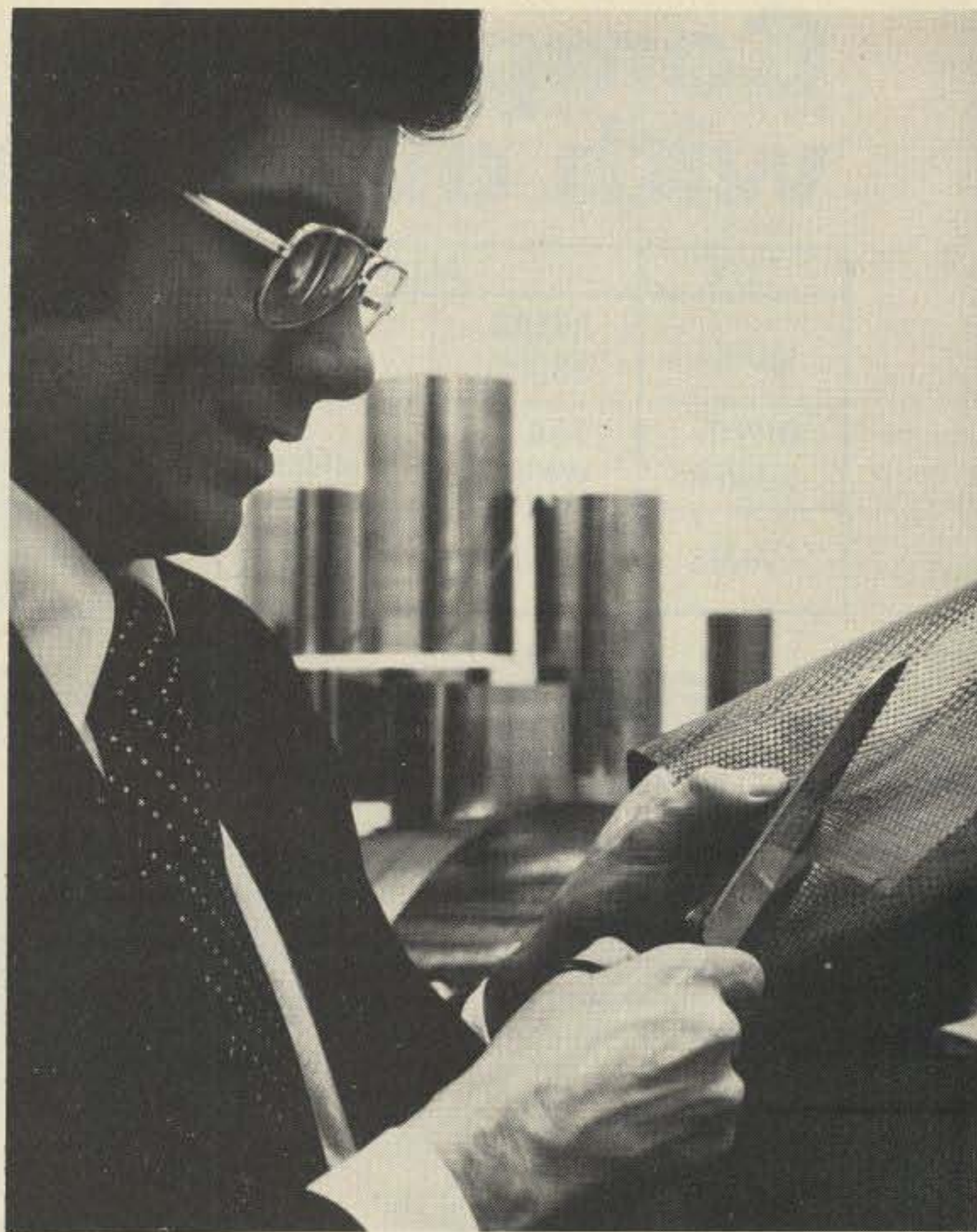
Greg Sellers, applications physicist, demonstrates the ease with which Metshield magnetic shielding fabric can be cut. Metshield fabric is the first commercial product made from Allied Chemical Corporation's Metglas amorphous metal alloys, a new kind of engineering material.
