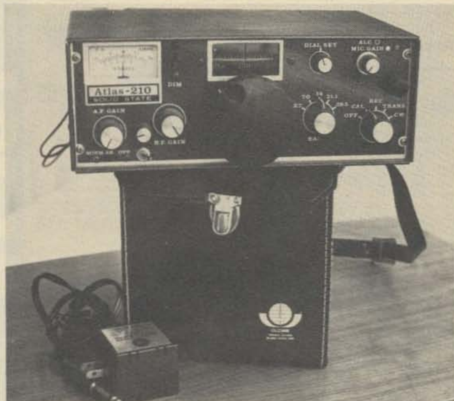
Fig. 1. A size comparison between a 210 and a Globe-Union battery pack which will power the unit at almost full power for several hours of intermittent operation.
