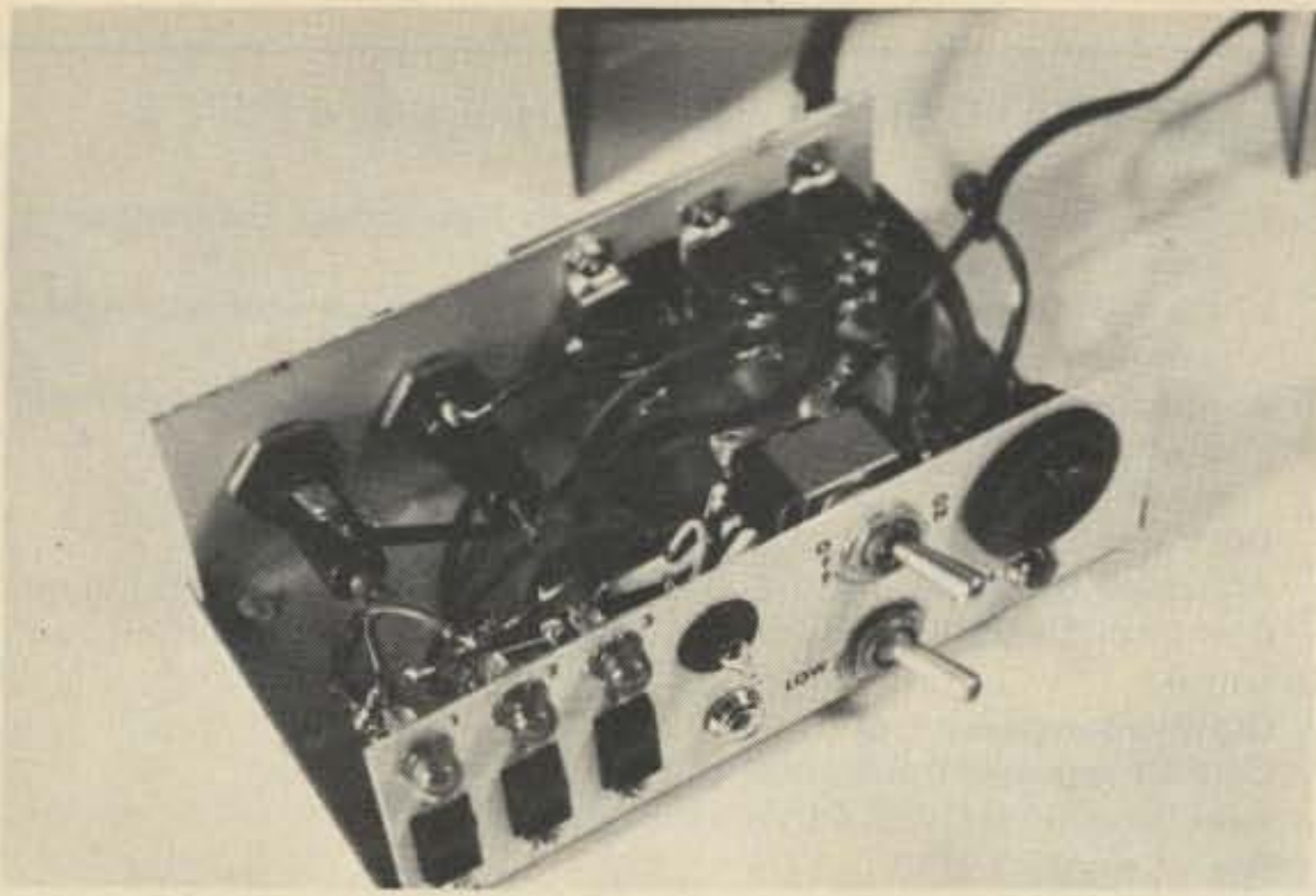
Internal parts placement should allow working space for top cover microswitch assembly. The light unit had its own power switch, eliminating the need for a switch on the chassis.
