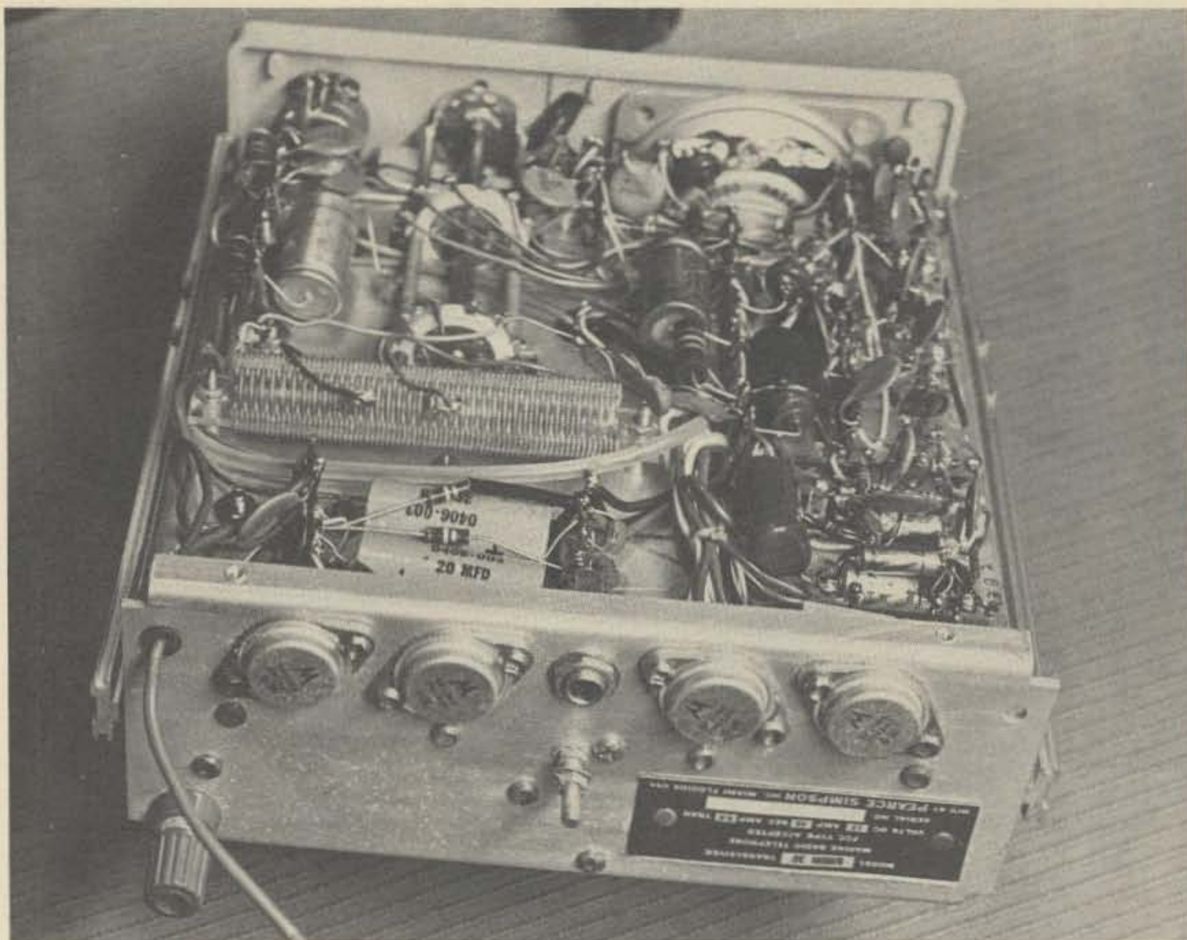
Fig. 3. Rear and bottom view of the BIMINI 30. From left to right across the rear panel are the modulator transistors, meter jack, B+ inverter transistors, 12 V dc lead and the antenna binding post. The final plate coil is seen beneath the chassis across the end of the channel selection switch.
