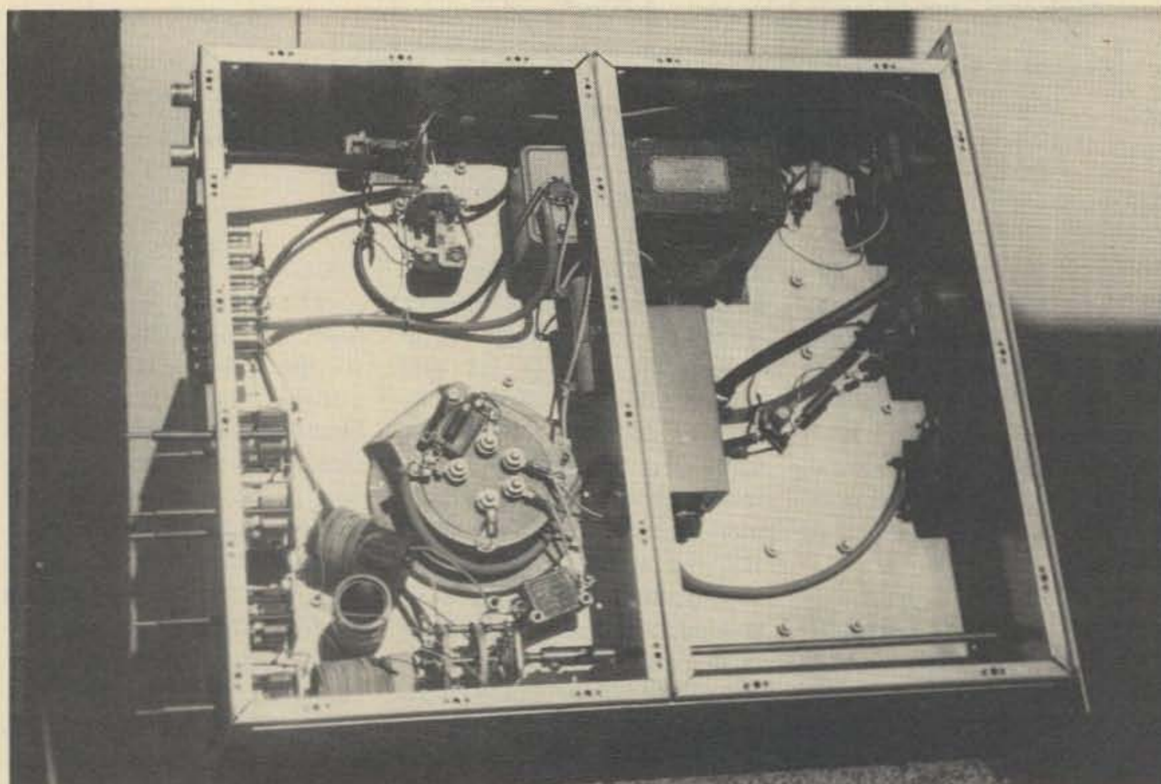
Bottom of chassis showing switching relays at top left, feedthrough filters and input tuning capacitors at left. The right half of the chassis contains the meters, filament transformer, and filament choke. Note the advantage of the two chassis arrangement for shielding.
