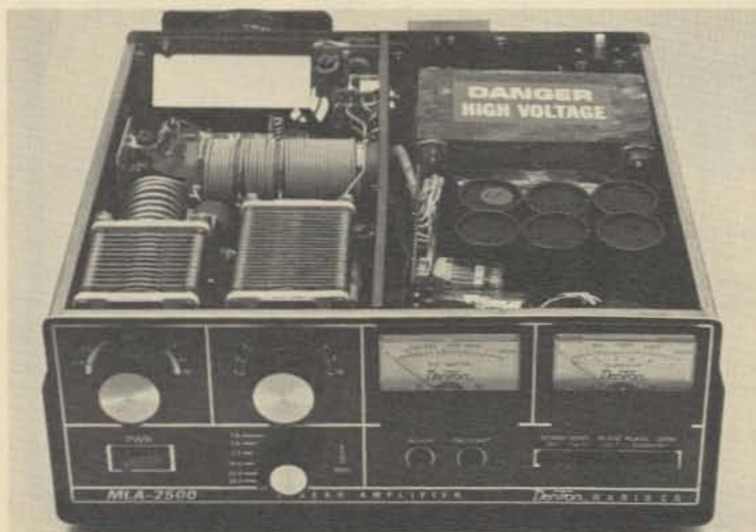
The Dentron MLA-2500 160-10m linear amplifier. The MLA offers modular construction, with a two step forced air cooling system.
