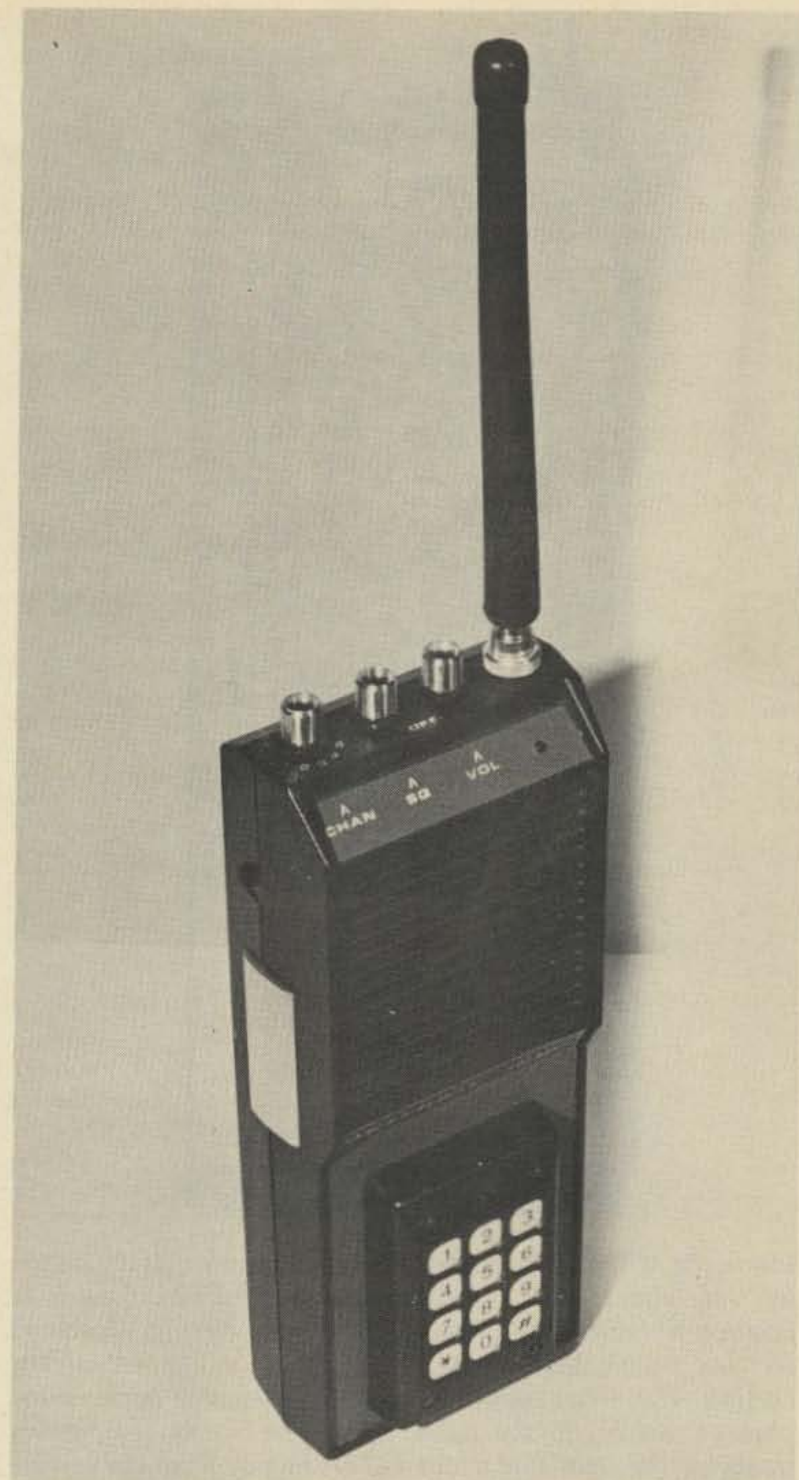
Heath HW-2021 2 meter handie-talkie with HWA-2021-3 autopatch encoder installed. Small slide switch above PTT bar on left side is the simplex/-600 kHz offset switch.
