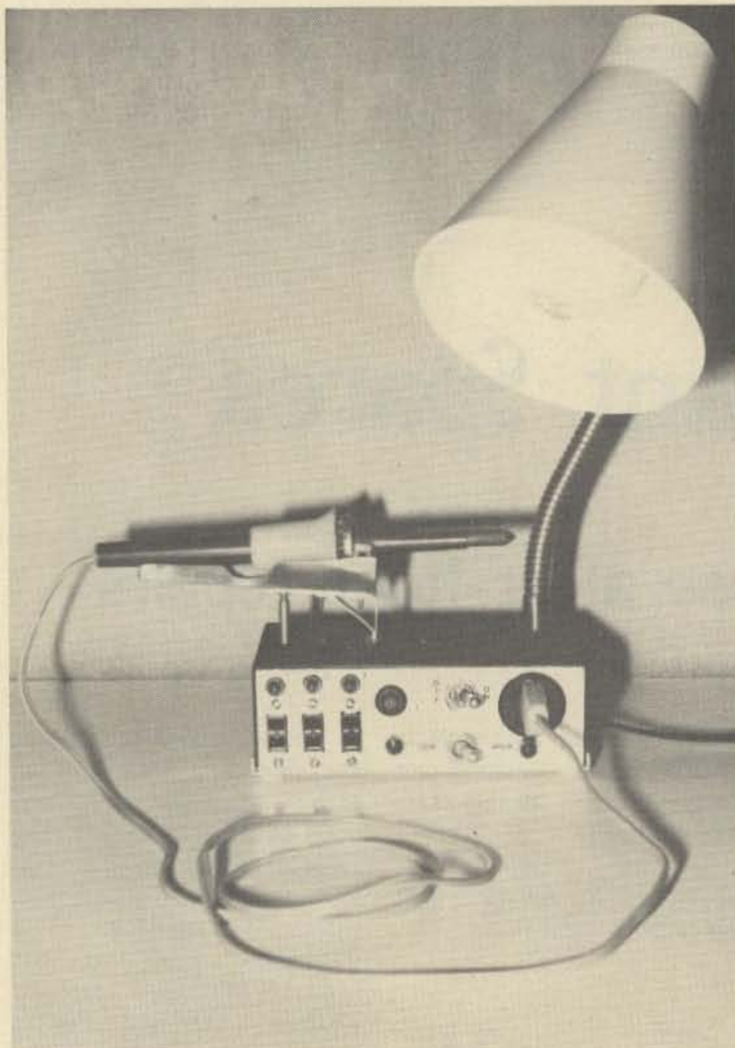
Workbench magic box with soldering iron in place and plugged in. Although the switches and fuses are on the rear panel, I elected to locate the indicator lights above the respective outlets. If the receptacle for the soldering iron was relocated to the left side panel, the cord might be easier to handle.
