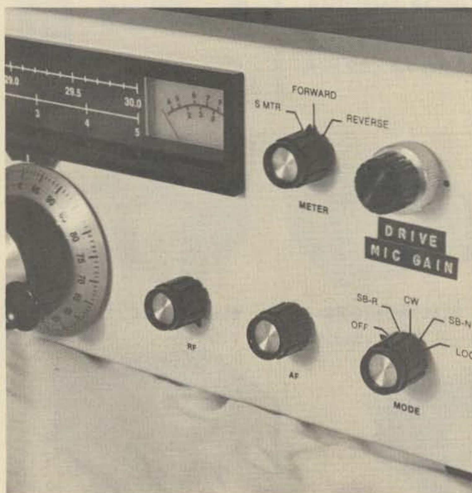
View of front panel after modification, showing new dual drive and mike gain control. The main tuning knob with spinner is the one used on the Triton IV and is a direct replacement for the Argonaut knob. The Triton knob is available from Ten-Tec for $1, postpaid.
