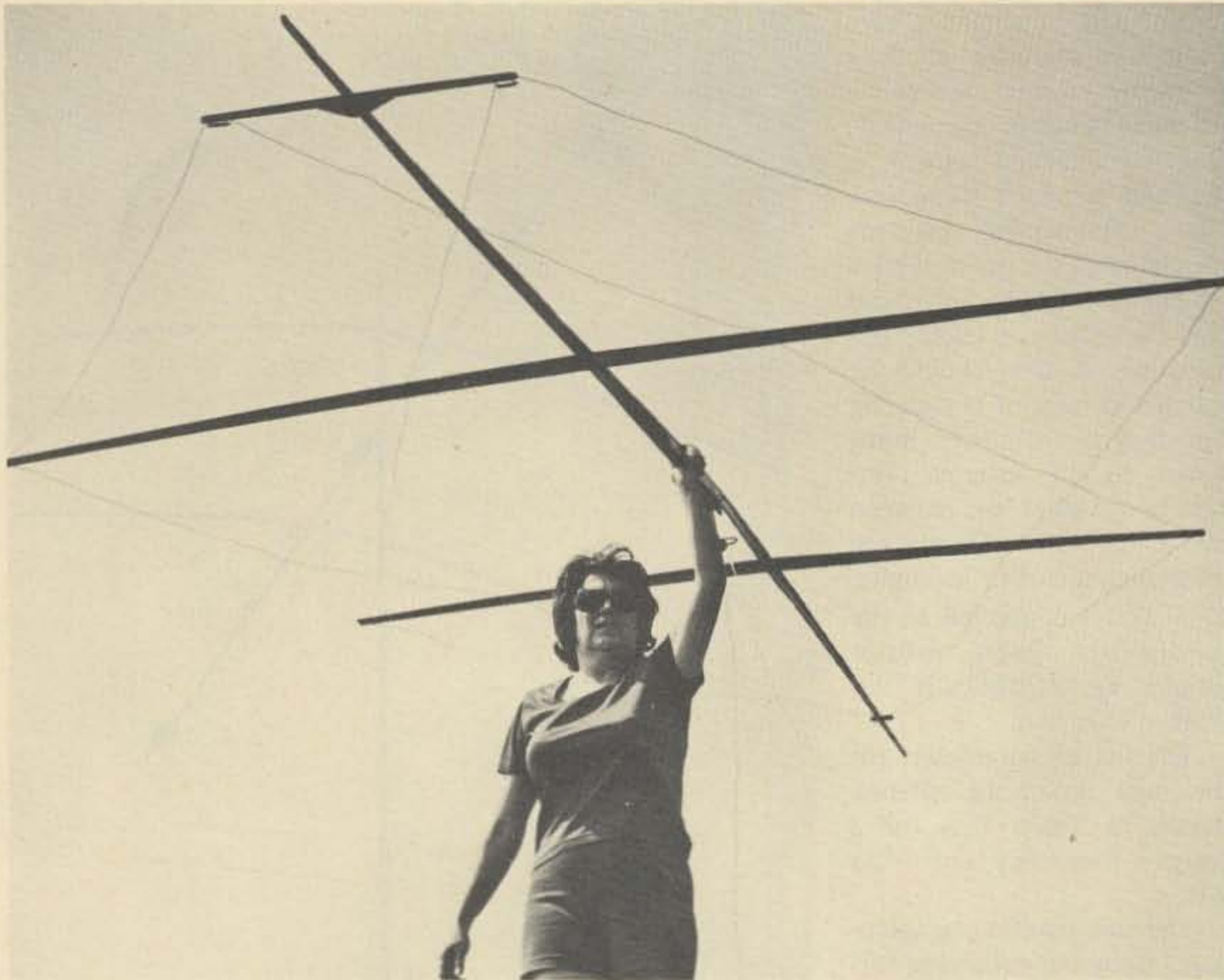
Dual rhomboid antenna held with one hand by W8DMR's XYL. Total boom length is 20'6".
