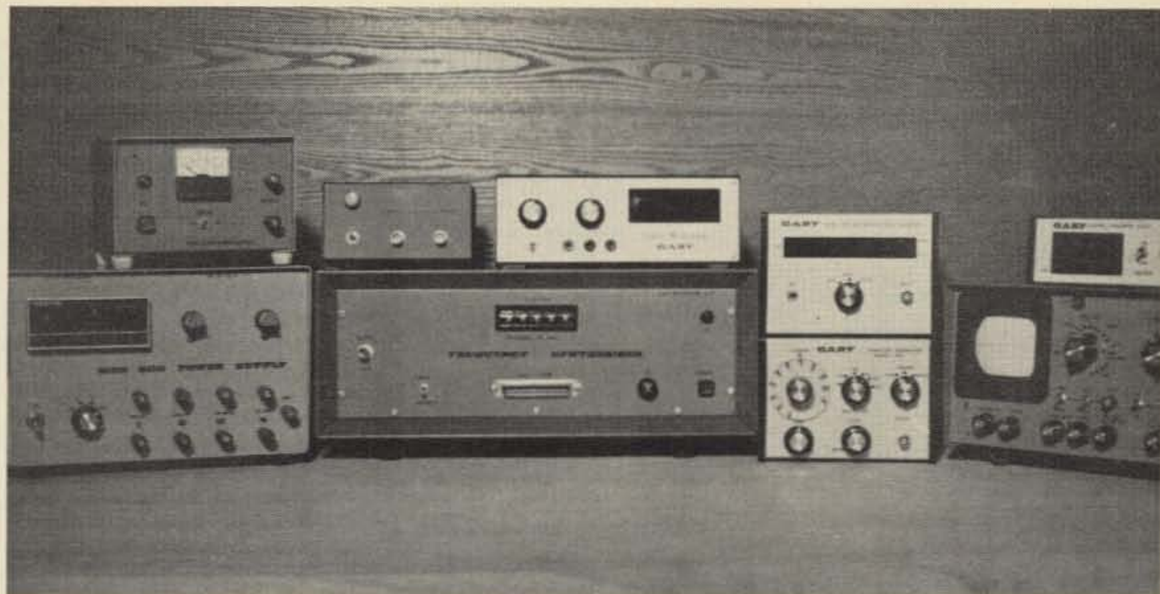
How would you like to sit down to a bench like this? This is part of the author's setup and all equipment is homemade. Shown from left to right are two stacked power supplies, a 0 to 60 MHz frequency synthesizer (signal generator), a frequency standard and digital multimeter on top, followed by a stacked function generator and counter. A triggered sweep oscilloscope is on the far right, and is topped by a digital alarm clock.
