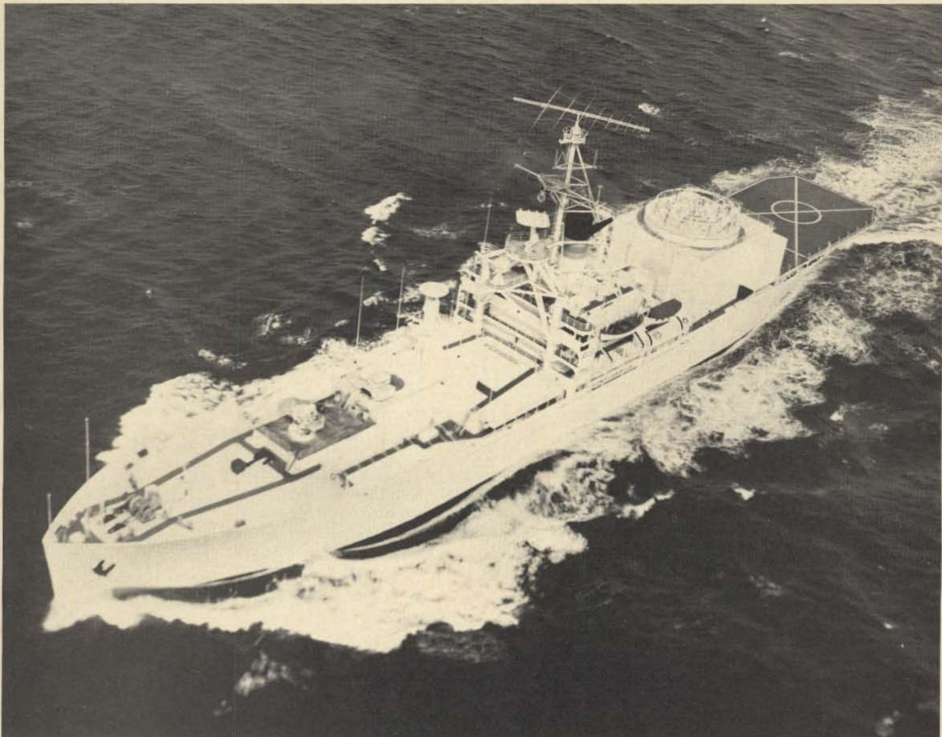
Fig. 2. The DDRR antenna is shown here installed aboard the U.S. Navy communications ship U.S.S. Wheeling. The antenna is seen mounted aft on the roof of the helicopter hangar. Operating efficiently even though exposed to the weather, the antenna was later covered with a pillbox fiberglass radome housing (official U.S. Navy photograph).
