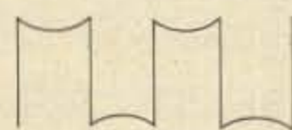
Fig. 2. Square wave after having passed through the notch filter.
