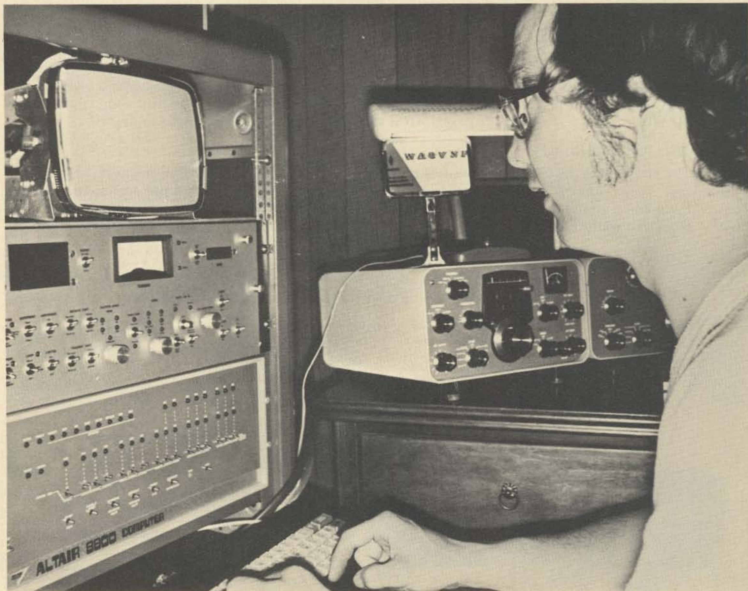
Station console. Computer, station control, video display, and keyboard are rack-mounted for ease of operation.
