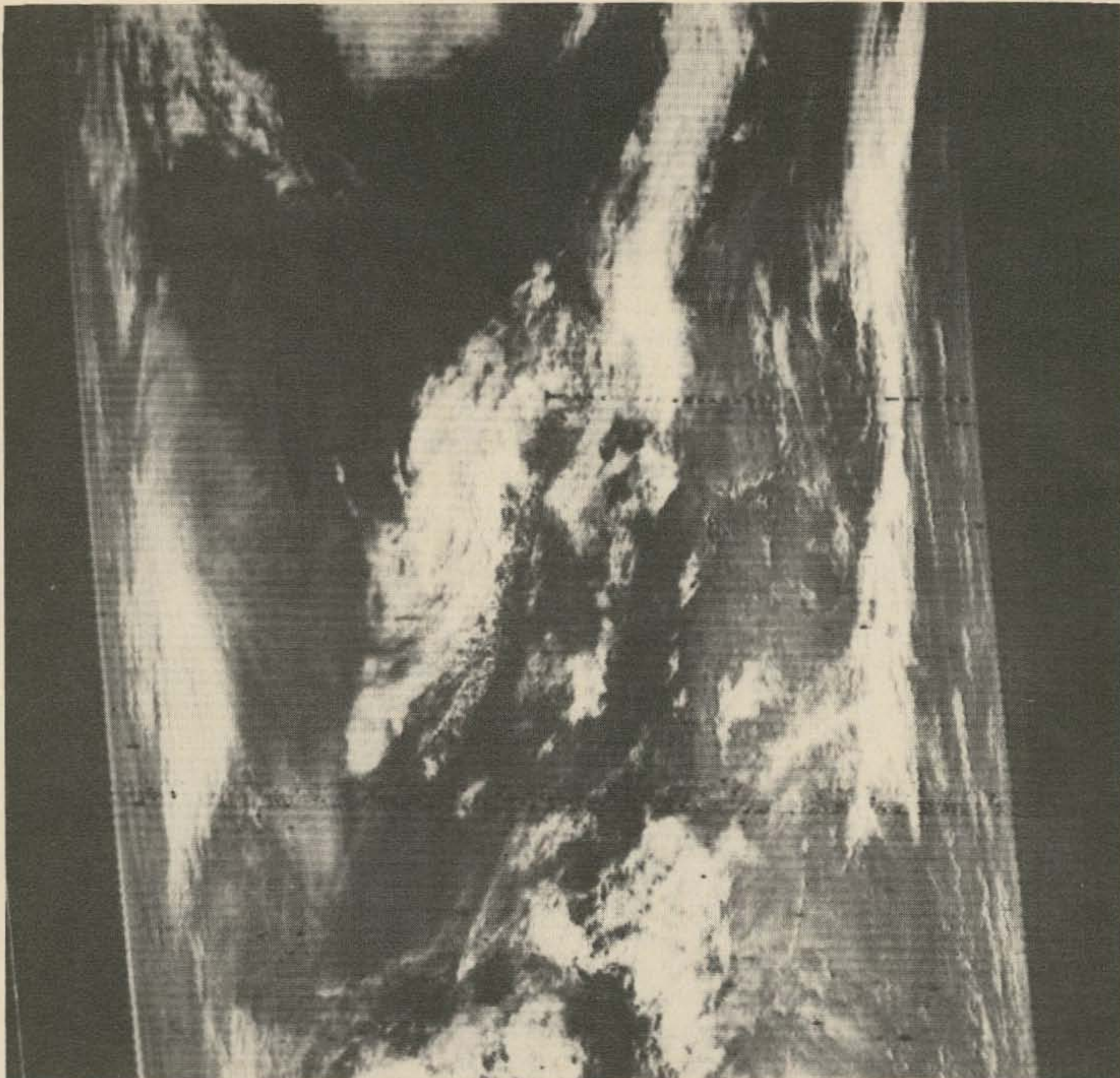
NOAA-4 visible channel view of the eastern U.S. on 13 May 1975. The original has a 4 x 6 inch format and was made using a rolling pin drum operating at 96 rpm (120 rpm motor on 48 Hz), with double the normal traverse motor speed for the drum size. Such larger format pictures present excellent resolution while minimizing the need for precision focusing of the light gun. The Great Lakes are visible just above and slightly to the left of the center of the picture.
