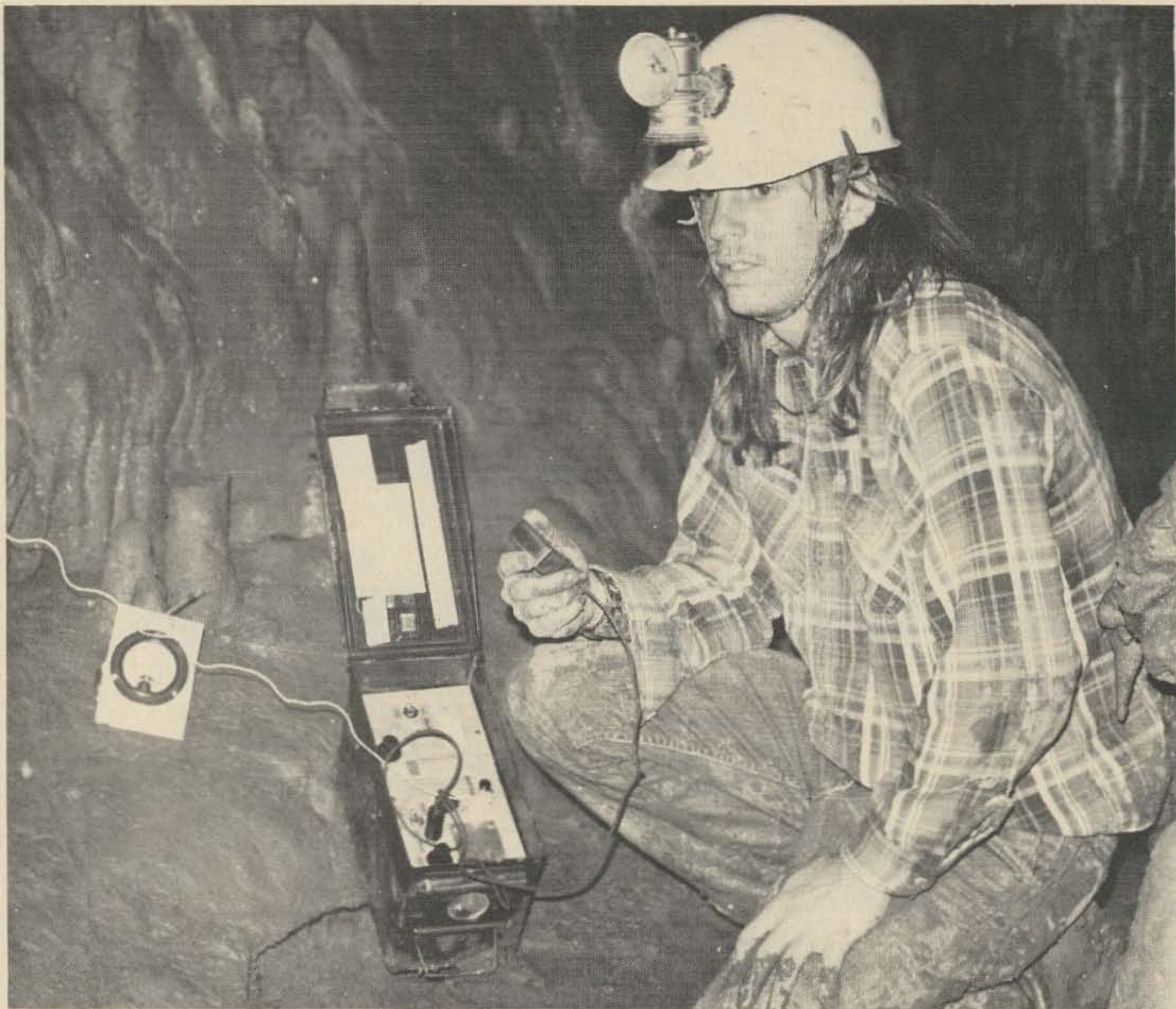
Operating KA2XAR mobile unit 1 in the depths of a wet, muddy cave is Bill Madden. He's operating on 1545 kHz, 10 W input, AM modulation. (Photo by James McCloud)
