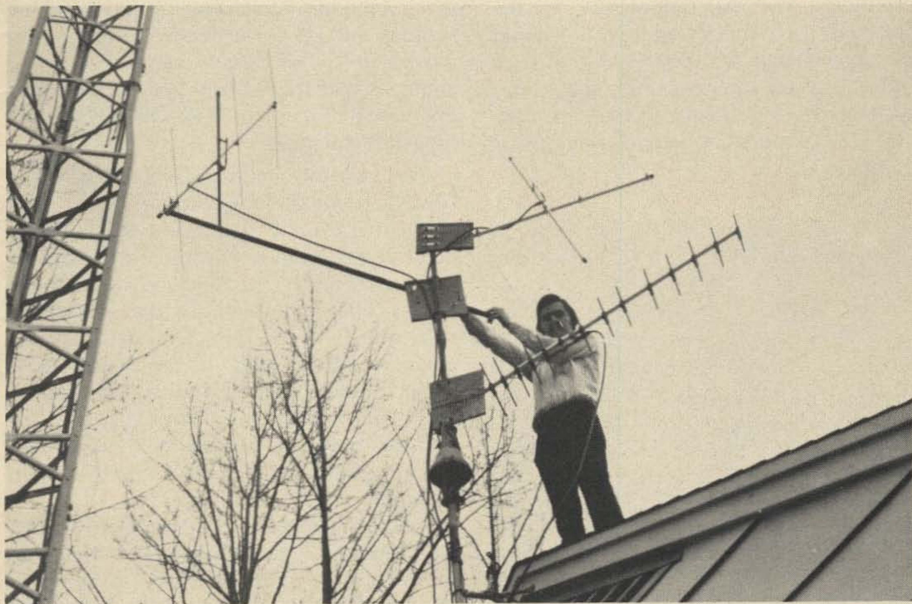
The author with his four element CushCraft two meter beams at 30 and 60. A fourteen element KLM beam for 432 MHz is used for AMSAT-OSCAR 7.
