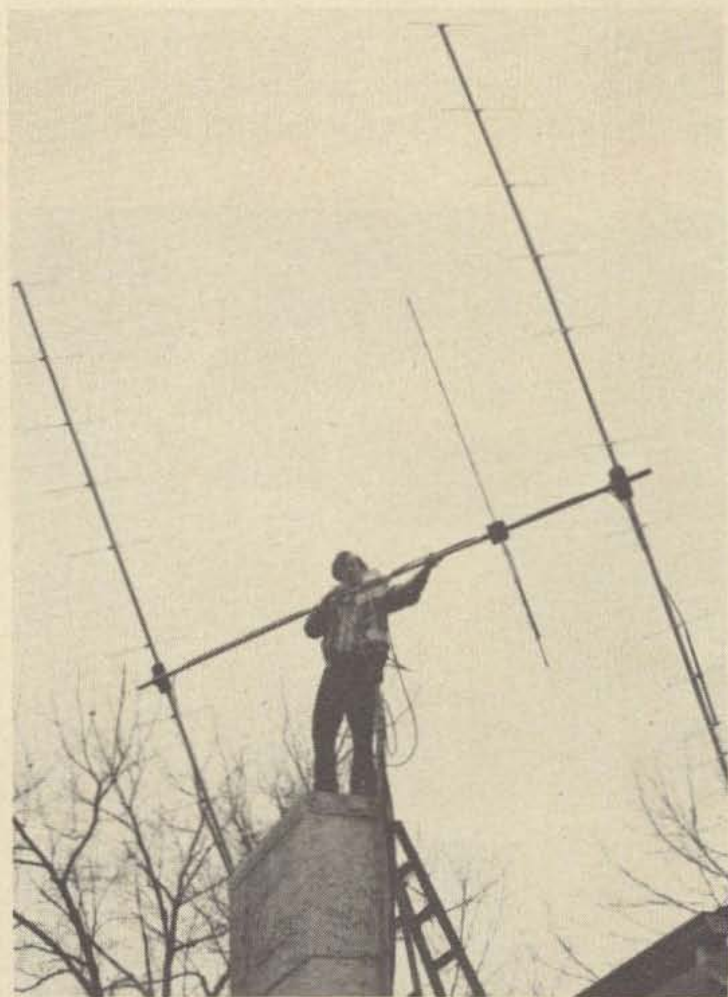
W3TMZ inspecting his AMSAT-OSCAR 7 antennas — two fourteen element KLM beams and a fourteen element 432 MHz K2RIW yagi.
