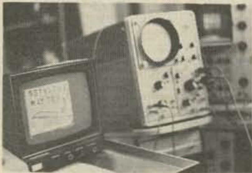
Here's the fast scan monitor at WB9LVI, displaying a slow scan picture through the aid of the slow to fast scan converter.
