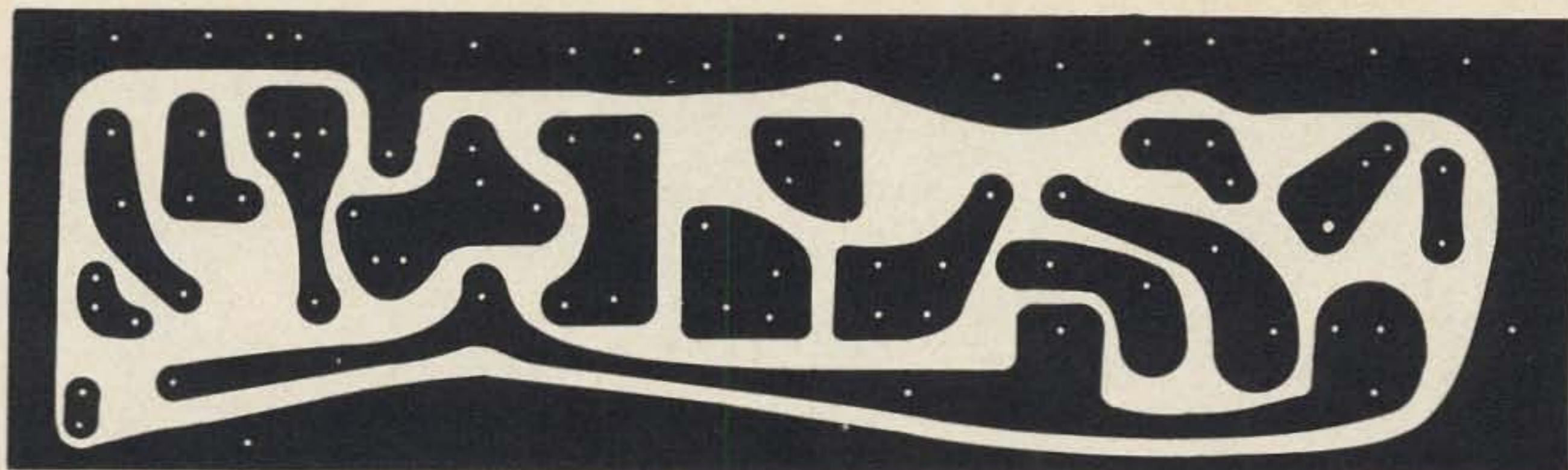
Fig. 4. Full size printed circuit VCXO board layout.
