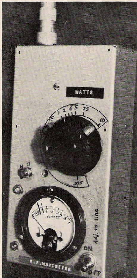
Top view of low powered rf wattmeter covering .025 to 10W. Built into a 8x4x2 chassis with wire screen bottom plate for ventilation.
