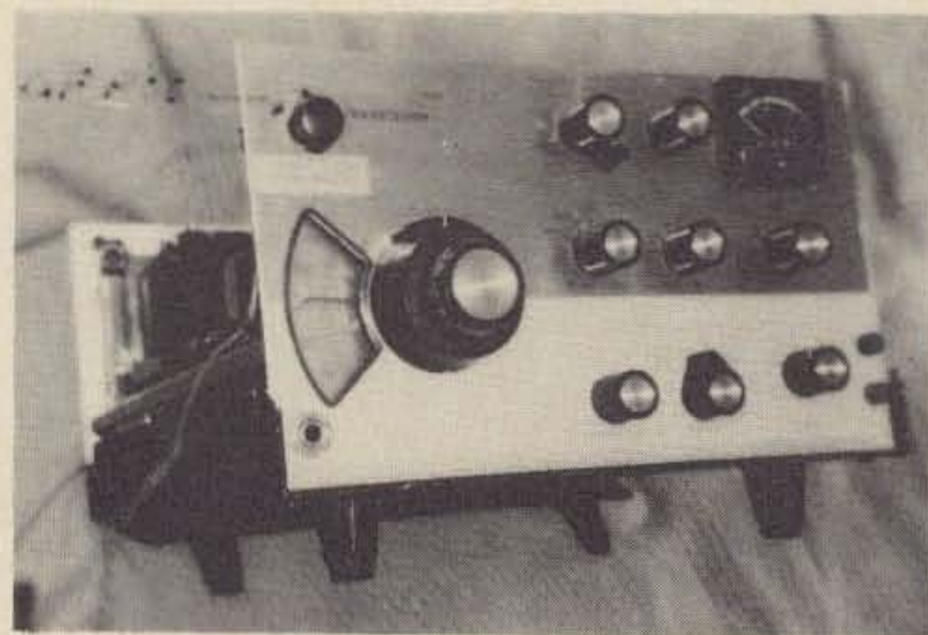
If you don't mind boring a small hole in the face of your transceiver you are sure to find a handy spot for the adjustment shaft. This one was placed in the upper left corner, right above the vfo dial.
