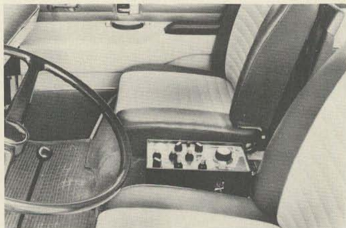
With the seat in place (covering the Drake's power supply), the power cables and antenna lead-in are out of sight. The microphone drops out of the way, too, and clips onto the side of the rig. (Probably the most important single consideration with any mobile setup is microphone cable routing. Lack of care in underdash rigs can lead to steering wheel entanglements and other such embarrassments.)
