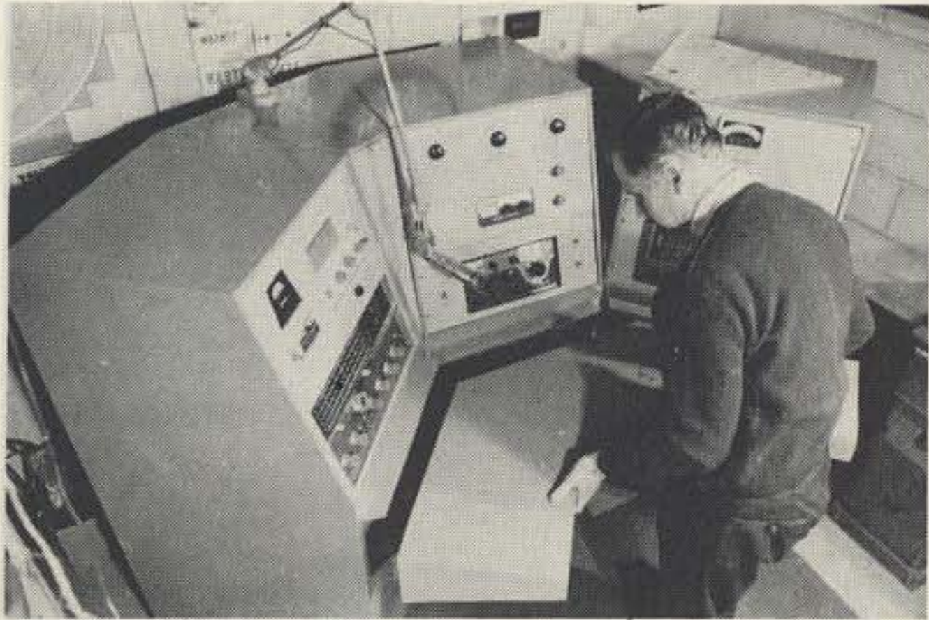
The desktop mounts neatly right over the support joists, locking the cabinets into a single three-bay console.
