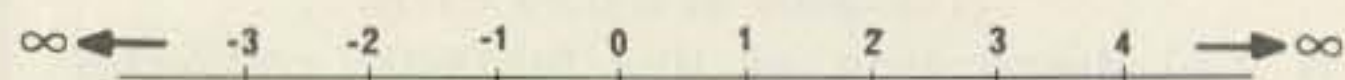
Fig. 5. This "number line" is basis of graphical method of determining impedance values. It provides conversion from picture to actual values.
