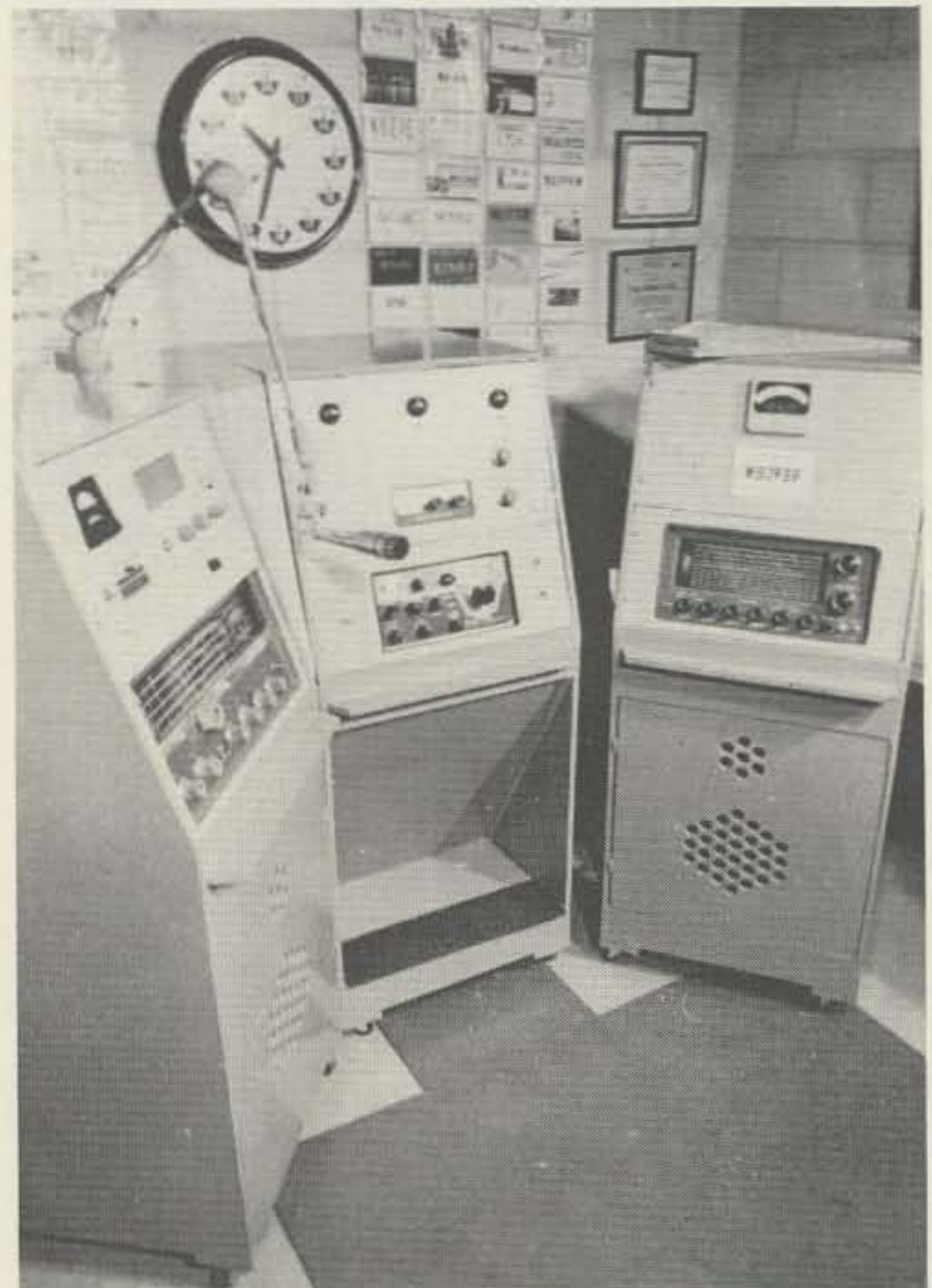
Removal of the tabletop and triangular "gap fillers" permits easy disassembly of the station for removal and transport. Note the "trailer hitch" connection between sections at lower right.
