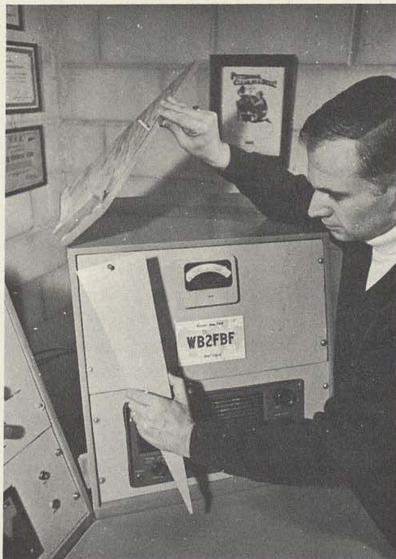
When the console bays are placed together, there will be large space gaps unless you build special-shaped wood sections like these. They add a professional touch and lend a look of uniformity to the three cabinets.
