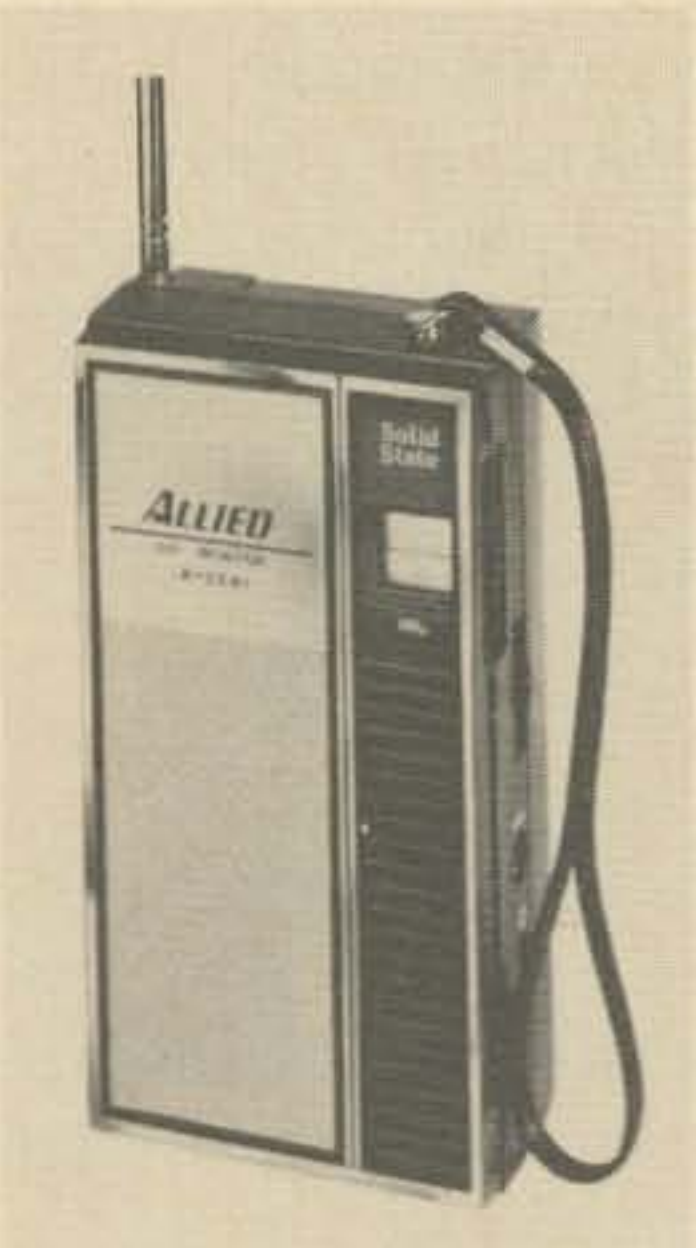
Fig. 4. Allied VHF monitor receiver is one of the first to include the FM portion of the 2-meter spectrum as part of its regular tuning range.
