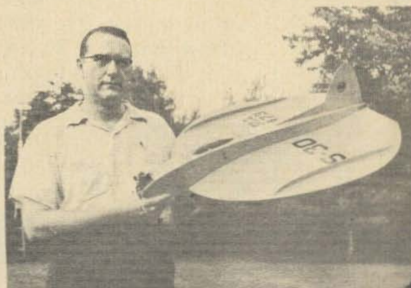
Seen one lately? This flying saucer is real. It is radio controlled and performs very well with a galloping-ghost proportional control system. This off-beat project was undertaken by W1OLP, writer of this article.
