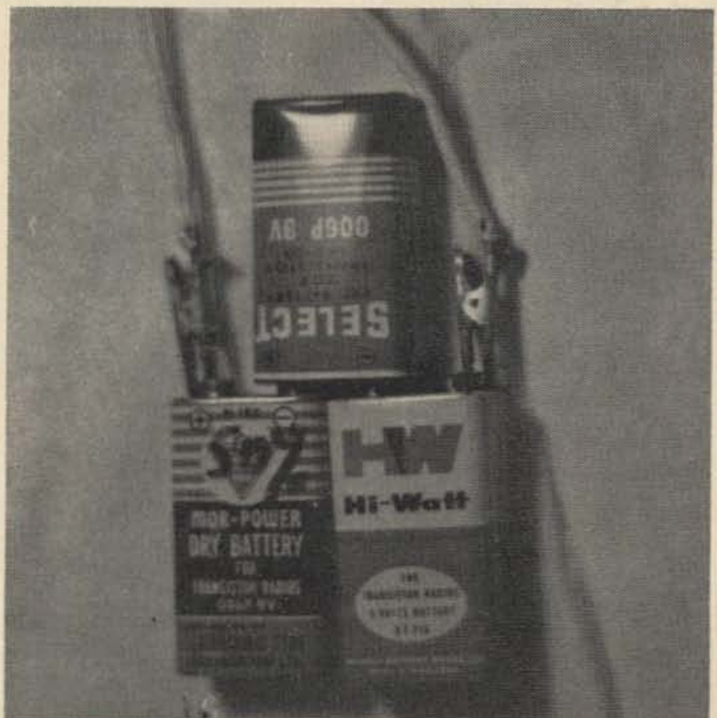
The series arrangement makes it easy to obtain odd voltages in increments of nine volts.
