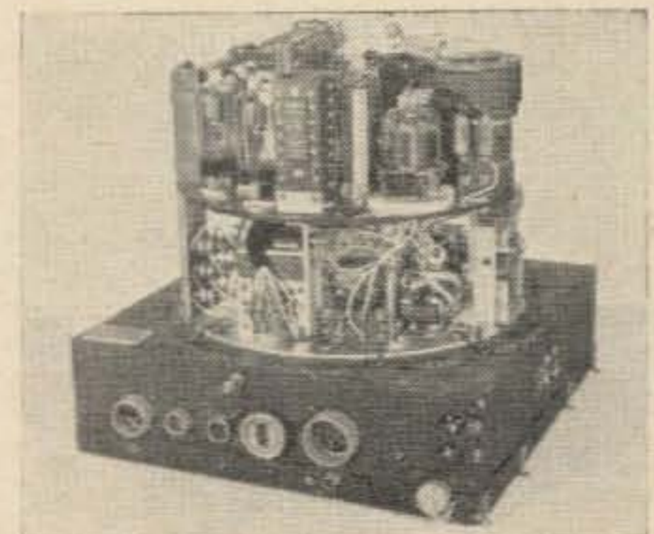
X-Band Radar An early airborne radar set for X band includes receiver and pulsed magnetron. Allow 100 lbs. $50.00 each. Here's your chance to have your own radar trap or weather eye. Requires 115V 400 cycles and 28V DC.
