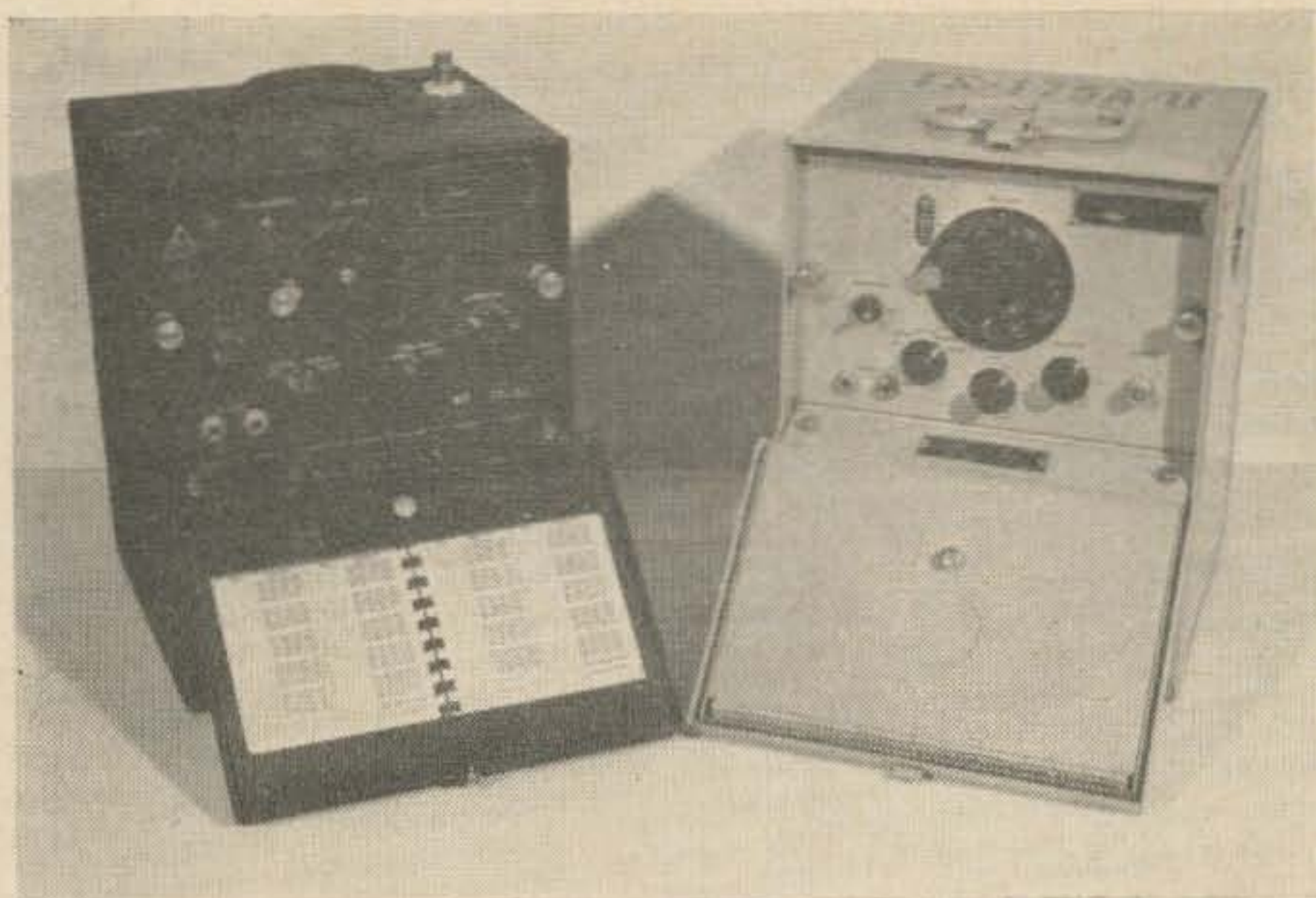
The unit illustrated at the right in the photo is the TS-175AU frequency meter. It is similar in operation and use to the BC-221, but covers a frequency range of 85 to 1000 mc. Price on it is $220.
