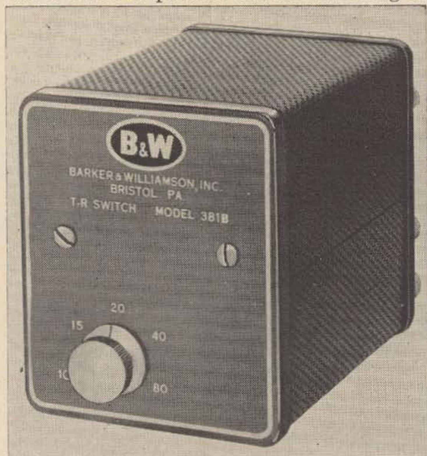
Photo courtesy Barker & Williamson, Inc. The B&W electronic T-R switch is an automatic unit that automatically switches the transmission line from receiver to transmitter when transmitting. This type of a switch is ideal for break-in operation and results in substantial receiver gain in most installations.
