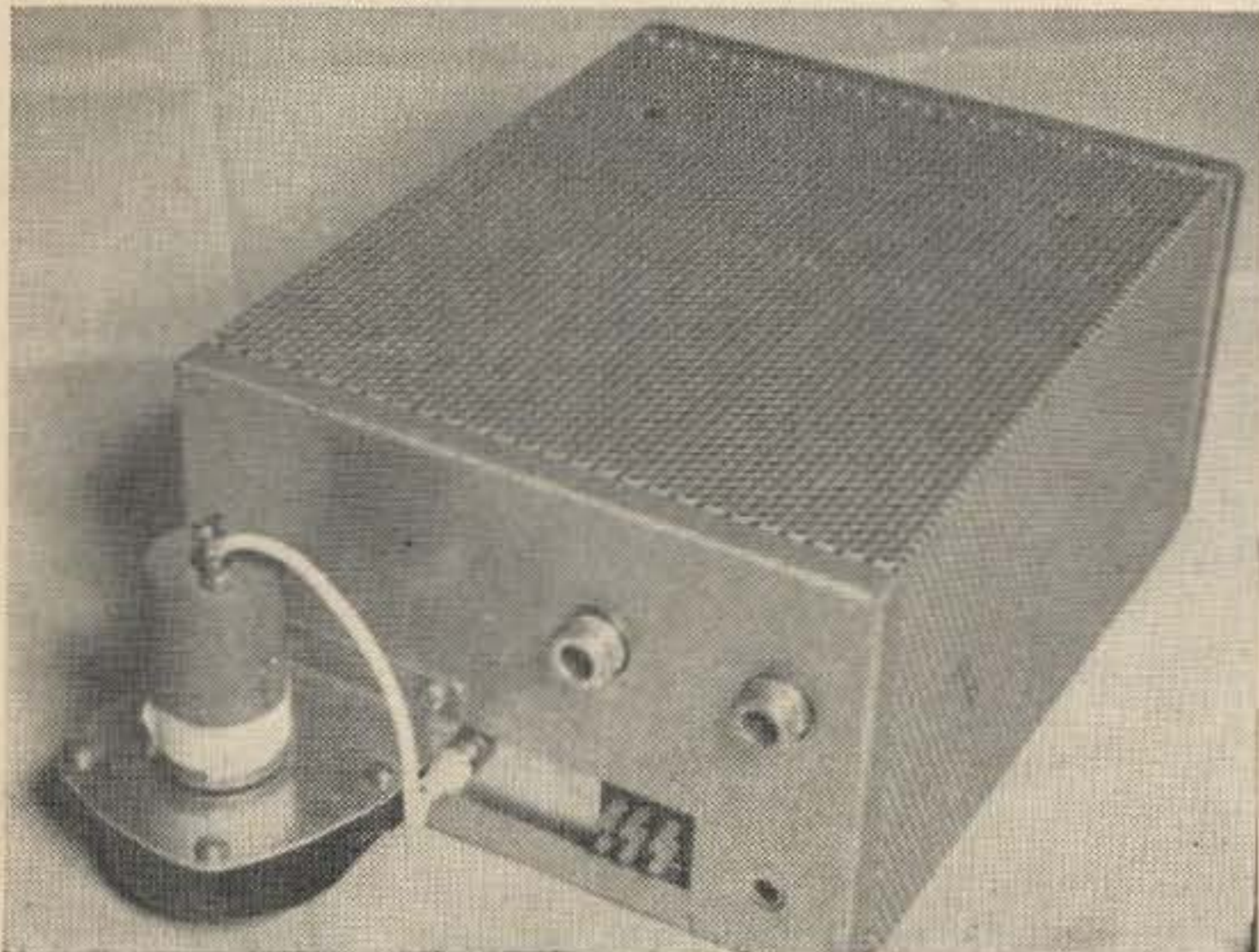
Back view of the transmitter showing the small blower, power receptacle, and the output jacks.
