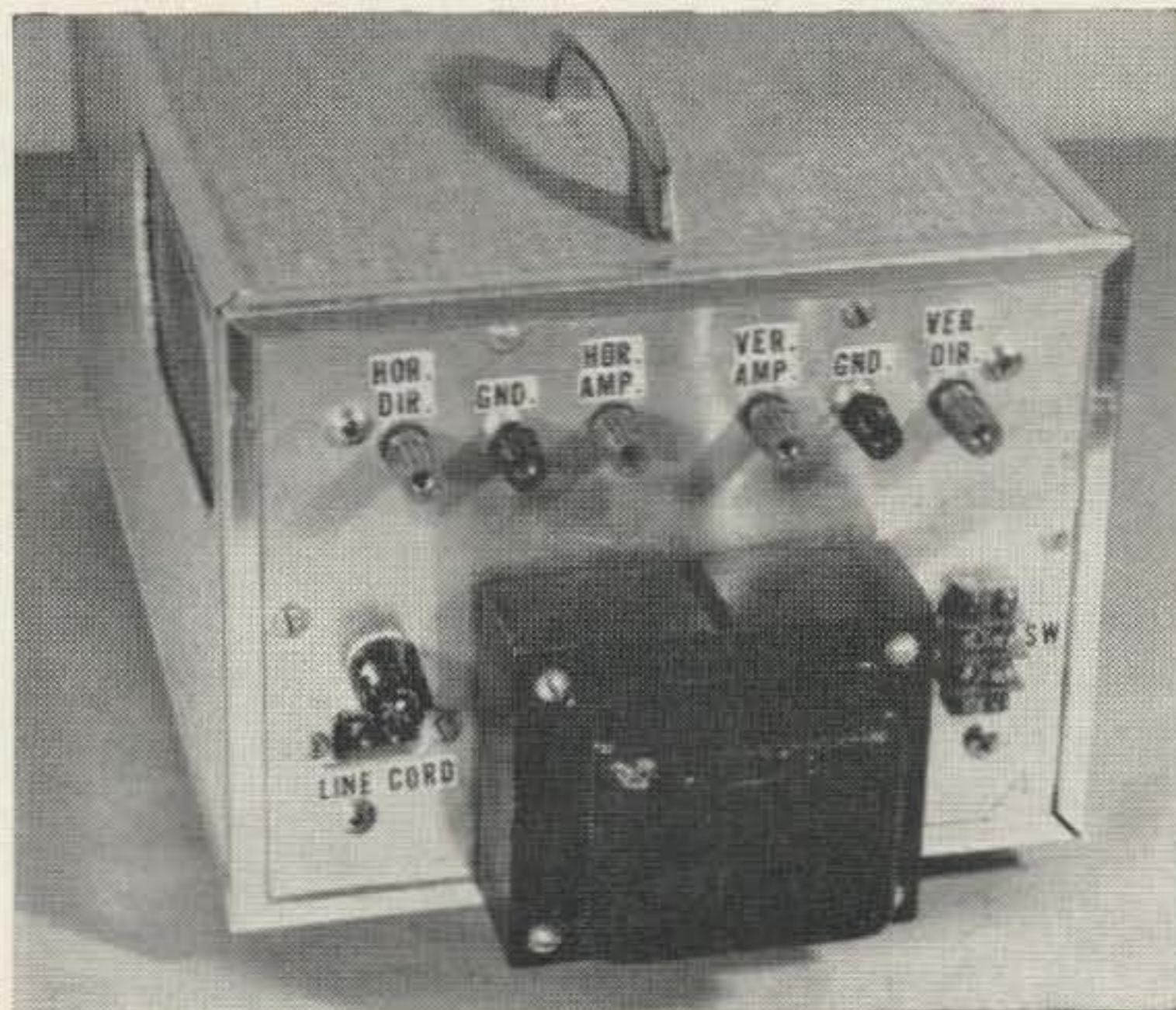
Rear view. Connections for remote control of spot to the right of transformer, fuse and ac connector on left. Input connections (3-way binding posts) across the top. Handle at rear top for balance.
