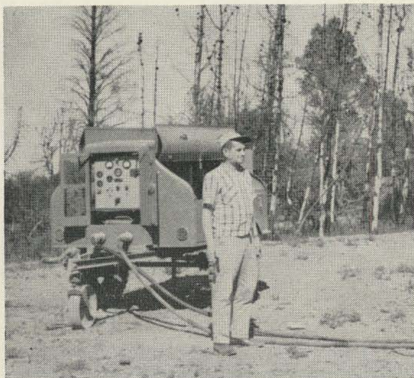
Tut WA6LUM inspects power cables from 7½ KW field day generator.
