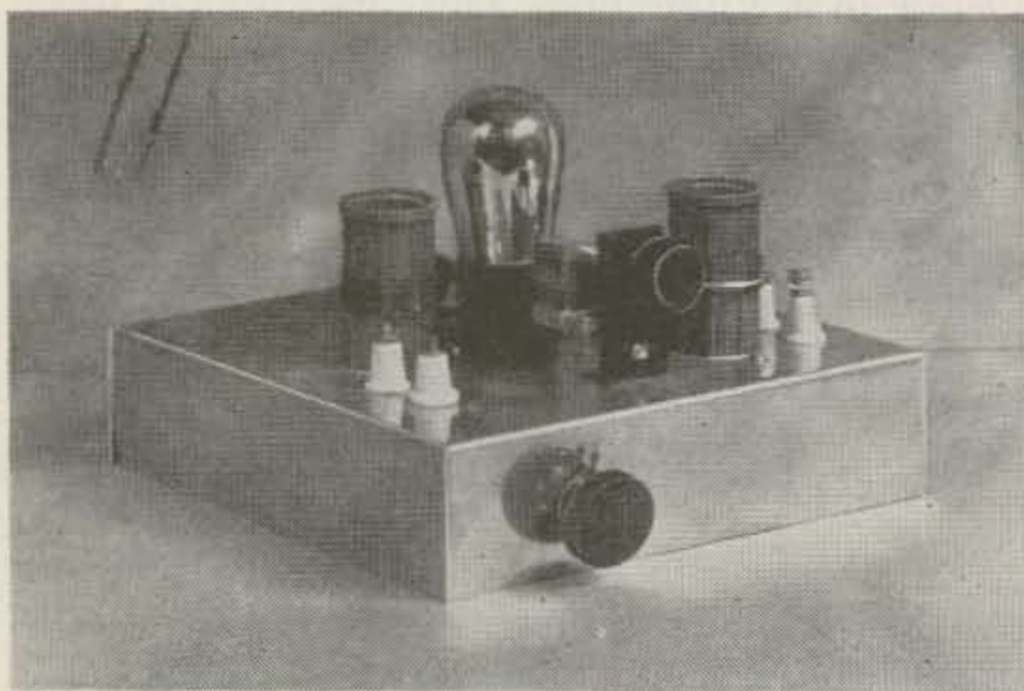
Tuned-plate, tuned-grid transmitter of the 30's. Grid coil on left, plate coil on right.
