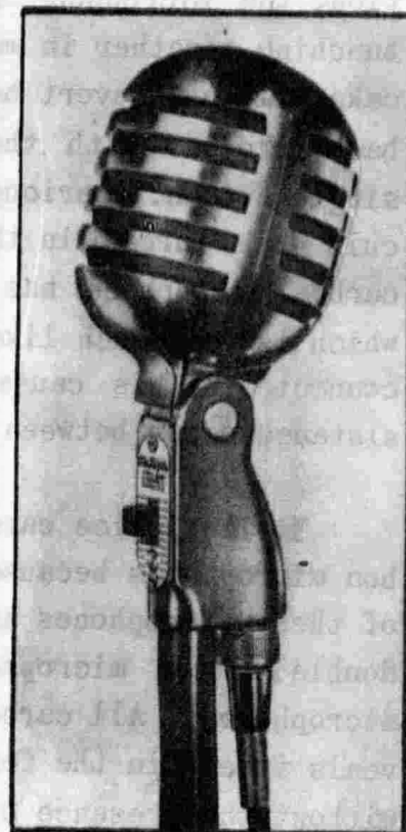
Fig. 8. Here is shown a photograph of a crystal microphone of the diaphragm type.
