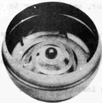
STATIC COLLECTOR INSTALLED IN FRONT WHEEL DUST CAP
