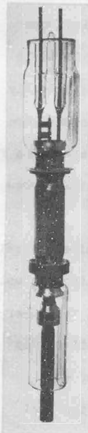
FIG. 2. A radio transmitting triode which is 40 inches high.
