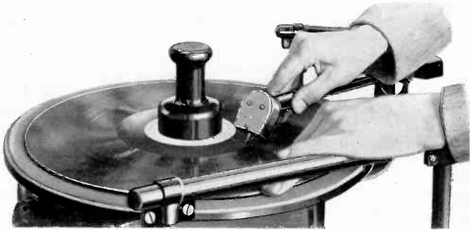
Figure 55—Placing a pick-up in the starting position for synchronous reproduction
