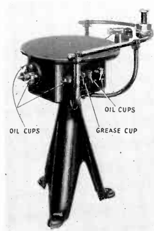
Figure 52—Type PT-7 synchronous turntable (Used in PG-10 equipments)
