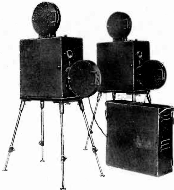
Figure 130—The projectors and amplifier used with the PG-5 portable equipment
