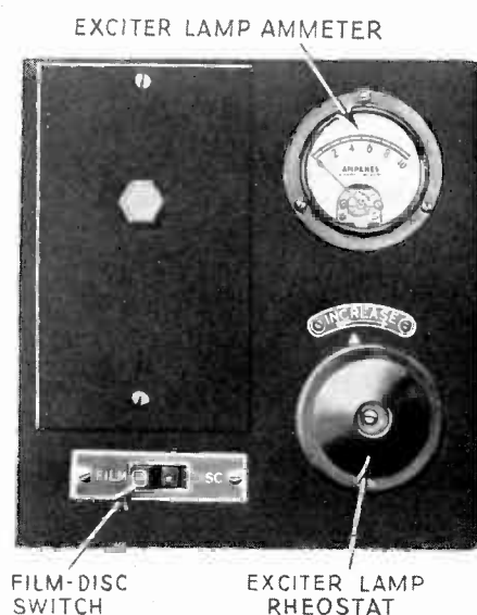
Figure 75—Photo-cell housing of sound heads used in PG-10 and 13 equipments
