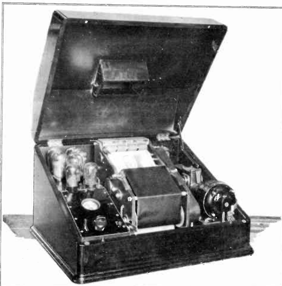
A SIX INCH CARBON RECORDER WITH ITS RECORDING AMPLIFIER AND SYNCHRONOUS DRIVE MOTOR
