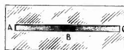
Fig. 3 - MORE OR LESS LIGHT REACHES THE PHOTOCCELL DEPENDING UPON THE OPTICAL DENSITY OF STRIP ABC.
