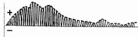
Fig. 6 - A CURVE DEPICTING THE ACTION WHEN THE NEGATIVE HALF OF A WAVE IS SUPPRESSED
