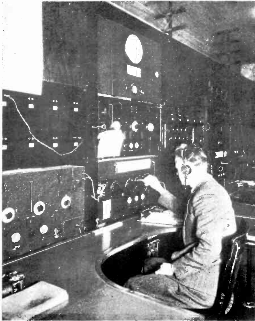
THE OPERATOR IN THIS PHOTOGRAPH KEEPS A SHARP WATCH FOR STRAYING FREQUENCIES AND IS SHOWN MANIPULATING MICROMETER TUNING CONTROL IN THE LABORATORY OF R.C.A. COMMUNICATIONS AT RIVERHEAD, LONG ISLAND.
