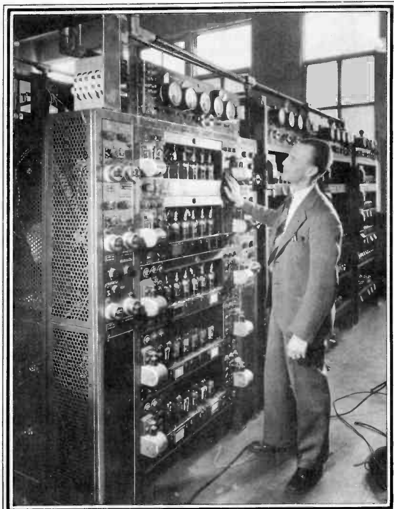
UNIVERSAL RACK FOR TESTING ALL TYPE RECEIVING TUBES UNDER VARIOUS VOLTAGE CONDITIONS
