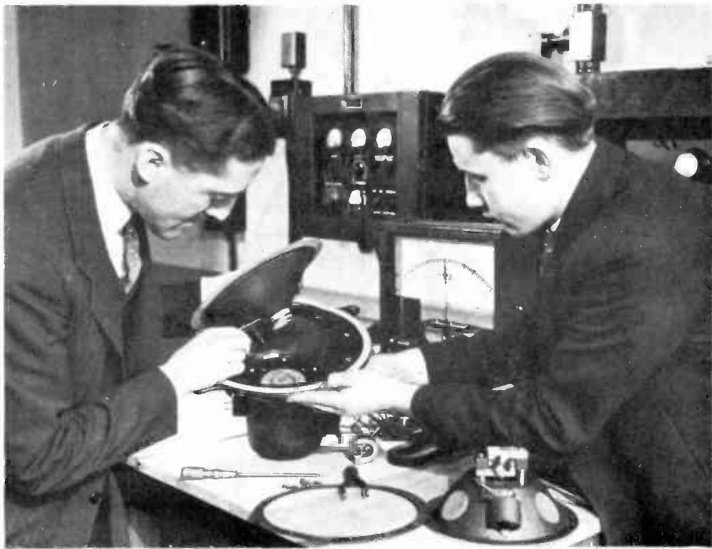
*The dynamic speaker being assembled depends on electromagnetic forces for its operation.*
