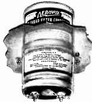
Showing inverted mounting with terminals on bottom of subpanel with unit partly above and partly below the subpanel.
