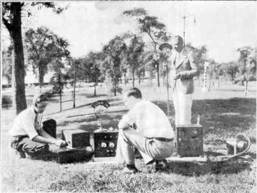
THE DYNAMOTOR AT THE RIGHT CONVERTS THE ELECTRIC POWER NECESSARY TO OPERATE THIS PORTABLE RADIO TRANSMITTER WHICH IS USED AS A FLEXIBLE LINK FOR TRANSMITTING SPORT AND NEWS EVENTS FROM REMOTE POINTS TO THE BROADCASTING STUDIO. (COURTESY COLUMBIA BROADCASTING SYSTEM)
