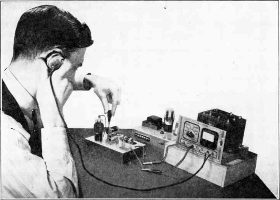
FIG. 27. If you arrange your beat frequency r.f. oscillator, power pack and N.R.I. Tester on your workbench in the manner shown here, there will be little chance for your hands and tester leads to affect the frequency of either of the r.f. oscillator circuits.
