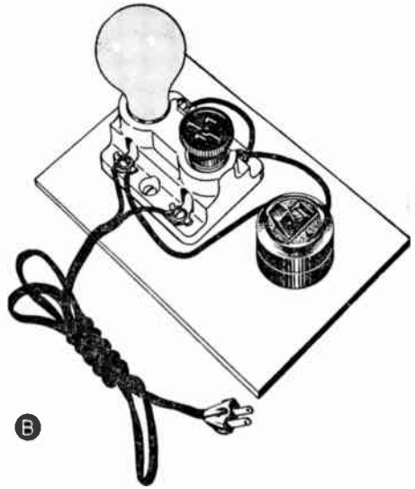
FIG. 5. A commercially manufactured heat control of the thermostat type is shown at A; one you can build yourself is shown at B.
