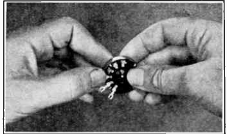
FIG. 35. Method of bending out the soldering lugs on the rotary selector switch (Part 2-6). Press them outward with your thumb, one at a time, until all the outer lugs point outward like the spokes of a wheel. Do not bend the single center lug.
