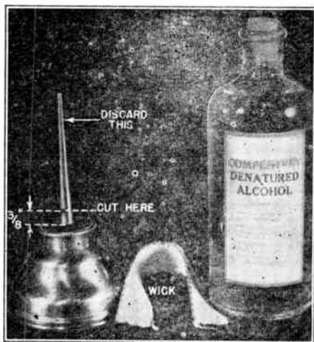
FIG. 7. Parts needed for making an alcohol lamp, which can be used for heating a plain soldering iron, for removing enamel from wires, and for heating an electric soldering iron in locations where power is not available.
