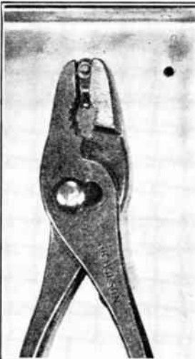
FIG. 24A. One method of using ordinary all-purpose pliers to prevent the soldering nut and lug from turning as screw is tightened.
