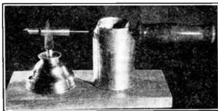
FIG. 8. Completed alcohol burner in use. The base is a wooden board of any convenient size. Three finishing nails hold the oil can in position on the base and prevent accidental tipping. A large empty tin can with notches cut in opposite sides can be used as a holder for the soldering iron, or you can cut a holder out of sheet metal for this purpose. The holder can be fastened to the base with two wood screws, in a position such that the copper barrel will be in the upper third portion of the flame.
