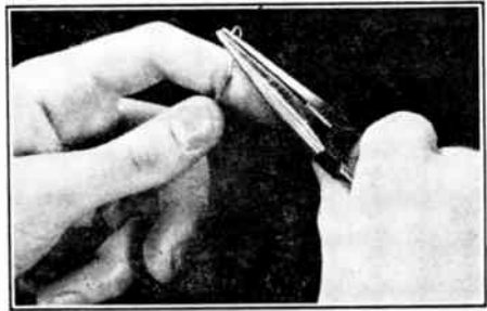
FIG. 27. Forming a hook on solid wire with long-nose pliers, preparatory to making a soldered hook joint.
