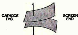
FIG. 16. Flared deflection plates of this sort are often used in electrostatic tubes.
