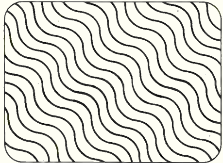
FIG. 8. Wavy lines show that the frequency of the interference is changing.
