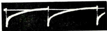
FIG. 27. Trace representing the wave shape at the grid of a vertical blocking oscillator.
