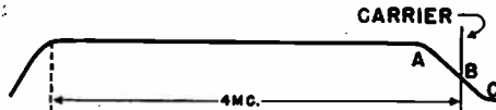
FIG. 4. Arranging the i.f. response so that the picture carrier falls at the point shown makes it possible to have a flat detector output and to pass all the desired side band with an i.f. band width of 4 mc.
