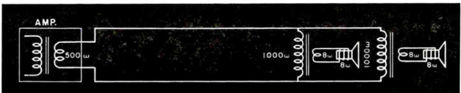
FIG. 17. Use of high-impedance line with separated loudspeakers.
