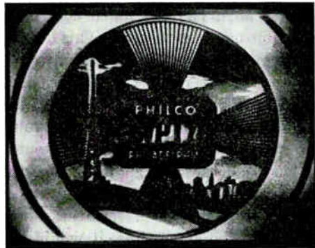
FIG. 21. The grid bias in this case is adjusted so that gray portions of the test pattern appear black, and we say the picture has too much contrast.
