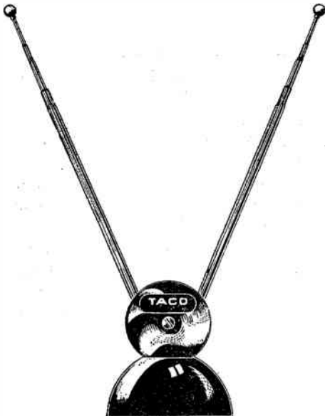
FIG. 26. A widely used form of indoor antenna.
