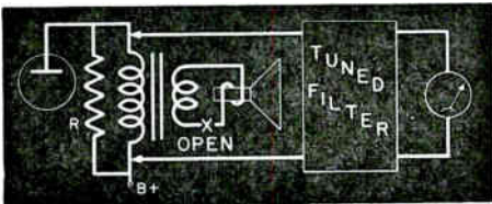
FIG. 15. A filter is necessary when measuring hum to eliminate noise components and to determine the amount of hum at each frequency. In practice, a serviceman would depend upon a listening test.
