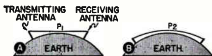
FIG. 1. The slight refraction of TV signals in air permits reception to be had over distances that are longer than the line-of-sight path.
