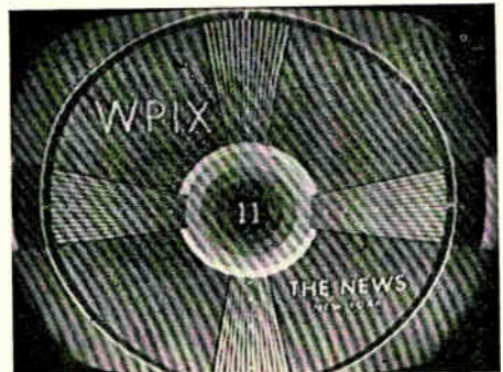
FIG. 18. Harmonics from an amateur or any other a.m. transmitter may produce regular lines of this sort. They will not change if the frequency of the transmitter does not change.
