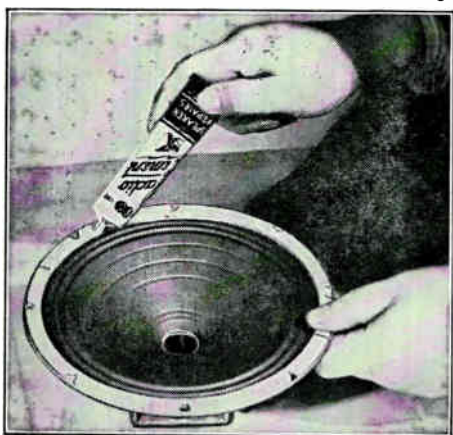
Applying speaker cement to a loose cone gasket ring.
