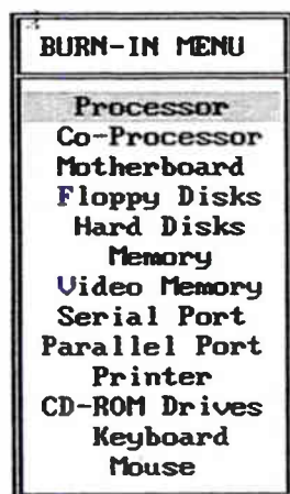
Figure 5. From the Burn-In Menu, you can select the tests you wish to perform during the burn-in process. It is also a good idea to run these tests as part of regular maintenance on the computer.
