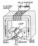
FIG. 6A. An a.c. generator in its simplest form has one coil of wire revolving in the magnetic field produced by an electromagnet.
