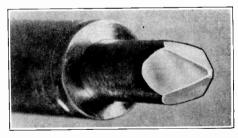
FIG. 8. Close-up photograph showing a properly tinned soldering iron tip. Note that only the flat surfaces of the copper tip are tinned.
