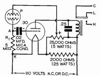
FIG. 17A. One form of the impulse circuit, using a selenium cell and a type 30 amplifier tube. The relay, normally closed, drops out when illumination on the cell is suddenly cut off. The relay remains pulled up for all constant values of illumination, and pulls up by itself at a definite time after each interruption of light.
