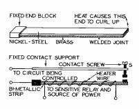
FIG. 12A. Basic principles of the bimetallic strip type time delay relay are illustrated here. The four connections shown to the relay are often reduced to three by attaching one heater wire to the bi-metallic strip.
