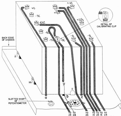
wire straight back along the chassis, then straight up along the side of the battery block, over the front corner of the block and back along the top of the block between terminals —A and —B. Push back the insulation and connect this wire to the  $+1\frac{1}{2}A$  terminal, then adjust its position as shown in Fig. 43.
