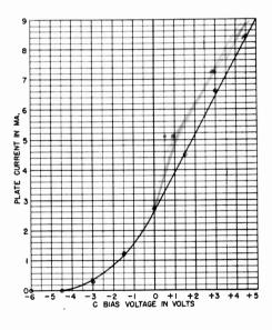
GRAPH 20C. Plot on this graph the results you obtain in Step 3 of Experiment 20, and connect the points together to give a smooth curve. This will be the characteristic curve of your type 1C5GT tube when operated as a pentode with a plate voltage of 45, a screen grid voltage of 22.5, and no plate load.
