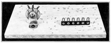
FIG. 24. For Step 1 of Experiment 28, mount the terminal strip and the potentiometer bracket in approximately the positions shown here, on a wooden base-board approximately 5'' wide, 7'' long and  $\frac{1}{2}$  thick.
