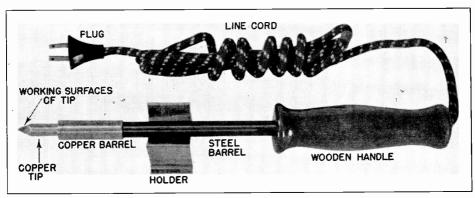
FIG. 3. Typical electric soldering iron for radio work. This is the soldering iron which is supplied to you as Part 1-1 in Radio Kit 1RK if you have access to 115-volt electric power. The correct way to use your soldering iron holder (Part 1-2) is also shown; the holder should be near to the copper barrel but should not touch it.
