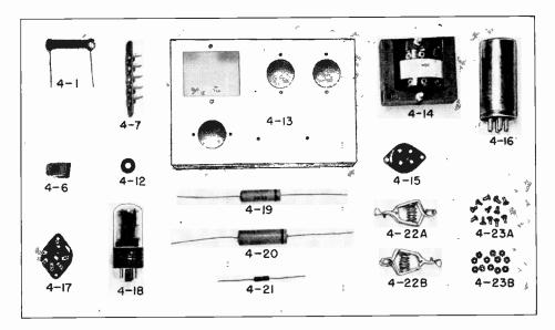
FIG. 1. The parts included in Radio Kit 4RK-DC are pictured above, and are identified in the list below. Numbers which are omitted from the part number sequence for 4RK-DC belong to parts which are included in the corresponding a.c. version of this kit and which have been replaced here by special d.c. power pack parts such as Parts 4-13 to 4-22. Some resistors may have a better tolerance (a lower percentage tolerance) than that indicated here.
