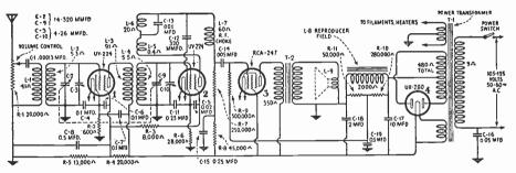
·Figure 1-Schematic Circuit Diagram of Model R-5
