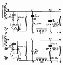
FIG. 31. Schematic circuit diagrams for Experiment 40DC, in which you duplicate the effects of dried-out electrolytic filter condensers by inserting an 18,000-ohm resistor in series with each filter condenser in turn and measuring the resulting a.c. filter input and output voltages.
