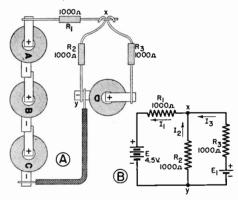
FIG. 13. Semi-pictorial and schematic circuit diagrams for Experiment 24.
