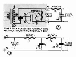
FIG. 27. Schematic circuit diagram for Experiment 38DC, in which you first connect one R-C filter to the output terminals of your power pack as shown at A while the power pack is connected as indicated in this diagram, then connect two similar R-C filters in cascade as shown at B.
