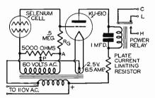
FIG. 21A. A practical photoconductive cell circuit, using a Westinghouse type KU-610 grid-glow tube to operate a power relay directly. Circuit operates entirely from A.C.
