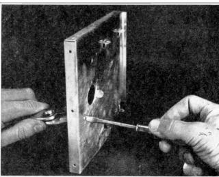
FIG. 21B. Another method of holding a nut with ordinary pliers while tightening a machine screw which is being used for mounting a soldering lug underneath the chassis. The screw should be tightened enough so that the lug cannot readily be moved with the finger.
