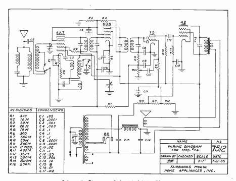
Schematic Diagram of the Model 56 Chassis
