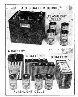
FIG. 2A (above). The only batteries you need for Experiments 11 to 20 in this manual and for the N. R. I. Tester are the four standard No. 2 (large size) flashlight cells and the special Burgess A-B-C battery block shown in this illustration. The A-B-C block contains a  $1\frac{1}{2}$ -volt A battery, a 45-volt B battery tapped at  $22\frac{1}{2}$  volts, and a 9-volt C battery tapped at -3,  $-4\frac{1}{2}$ , -6 and  $-7\frac{1}{2}$  volts.
