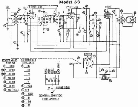
Figure 4—Schematic Wiring Diagram
