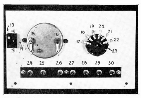
FIG. 37. The back of your tester panel should appear like this after you have mounted the selector switch and ON-OFF switch, as instructed in Steps 2 and 3. (The meter and jack strip were mounted as part of Experiment 11.) Number the various terminals on your own panel by marking them with crayon or pencil as shown in this view. Crayon markings can be wiped off with a cloth if errors in numbering are made.
