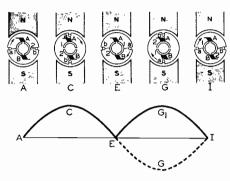
Fig. 8B. Output voltage curve for a simple d.c. generator.
