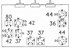
F = Filament SG = Screen GridP = Plate CG = Control Grid
