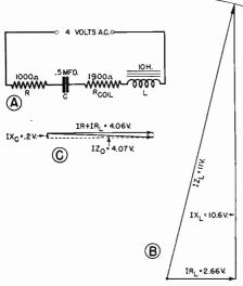
FIG. 31. Equivalent simplified circuit diagram corresponding to Fig. 30B, and vector diagrams which prove that Kirchhoff's Voltage Law for a.c. circuits holds true in this particular circuit when tested out with the values obtained in the N.R.I. laboratory. One volt on these diagrams corresponds to ½-inch of vector length.
