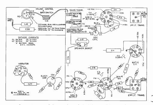
Bottom view-rear of chassis. Radiotron Socket Voltages, and Location of parts
