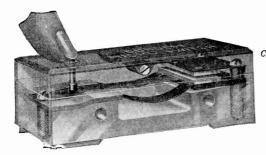
Courtesy C. F. Burgess Laboratories, Inc. FIG. 9A. Phantom view of the Burgess micro-switch. A slight pressure on the plunger at the left either opens or closes the silver contacts at the other ends of the spring steel blades, depending upon how the contacts are arranged.
