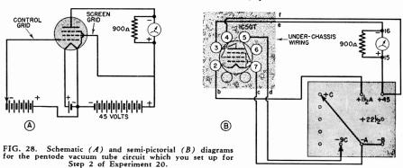
from chassis hole d (this lead is shown on +C in Fig. 23B). Read the meter on scale  $I_{\rm M}$ , and record your results (both the meter reading and the actual current in ma., which is three times the meter reading) on the first line of Table 20A as the plate current for a C bias voltage of -9 volts.
