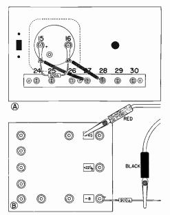
FIG. 15. By placing a 100-ohm shunt resistor across your meter in the manner shown at A here, you are able to measure (Experiment 15) the current in the circuit shown at B, even though this current is considerably higher than the 3-ma. maximum value which can be passed through the meter alone.
