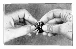
FIG. 35. Method of bending out the soldering lugs on the rotary selector switch (Part 2-6). Press them outward with your thumb, one at a time, until all the outer lugs point outward like the spokes of a wheel. Do not bend the single center lug.
