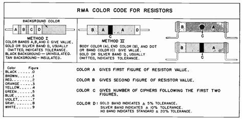
FIG. 3. The two methods being used for marking resistors according to the standard R.M.A. Color Code are given here.
