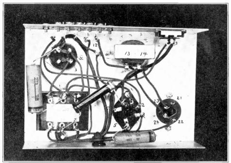
FIG. 9. Your vibrator power pack should appear like this under the chassis after all wiring has been completed.
