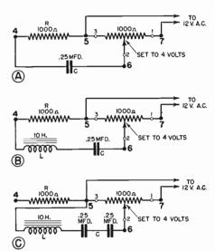
FIG. 18. Schematic circuit diagram for Experiment 29DC.
