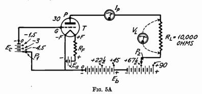
can be changed, and in this simple experiment the connections to batteries  $E_{\rm c}$  and  $E_{\rm b}$  may be changed. Dotted lines ending in arrows usually indicate that the connection is only temporary, or in this case for the purpose of measuring voltage only when desired.
