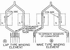
Fig. 9. Types of winding elements.
