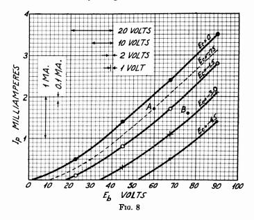
mined from this figure and the family of curves given in Fig. 8, if we are willing to employ a little elementary arithmetic, such as is taught in the primary and grade schools. Although you will rarely have to compute anything when servicing a radio receiver, I will have to make simple calculations in these lessons in order to make clear certain ideas that I want you to understand.
