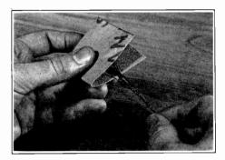
FIG. 16. Method of using fine sandpaper (about Number 00) to remove enamel from stranded wire. Press the folded sandpaper (about one inch wide and two inches long) together with the wire in between as indicated, then draw out the wire. Repeat until the enamel is entirely removed from the portion of wire which is to be soldered.
