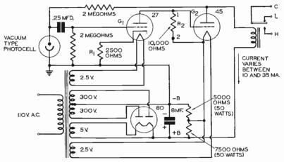
FIG. 18. Typical two-stage amplifier circuit for a vacuum type photocell connected into an impulse circuit; the type 80 tube supplies full-wave rectified D.C.
