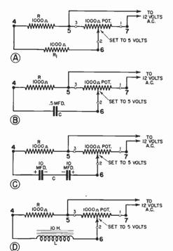
FIG. 15. Schematic circuit diagrams for Steps 5, 6, 7 and 8 in Experiment 28DC.
