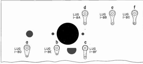
FIG. 23. Upon completion of Experiment 5, you should have the six soldering lugs, all tinned, mounted on the chassis exactly as shown here, with the ends of the lugs bent upward as shown in Fig. 20.
