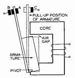
FIG. 8. Diagram illustrating the principle of operation of the minimum reluctance type of power relay. Dotted lines show pull-up position of armature.
