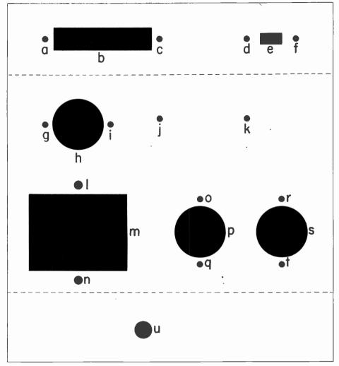
FIG. 3. Chassis layout diagram for the d.c. power pack, drawn to show what you would see if you looked at the bottom of the chassis while it was a flat sheet (before bending the sides). The dotted lines indicate the positions of the bends. The holes are lettered here merely for your convenience in locating on your own chassis the correct mounting holes for the various parts; do not mark the holes in this manner on your chassis, for this diagram is entirely sufficient for assembly purposes.
