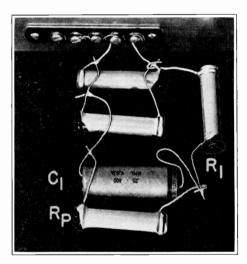
FIG. 30. Suggested method of connecting to the d.c. output terminals of your power pack a 20,000-ohm load and an arrangement of two resistors and a condenser  $(R_1, R_P \text{ and } C_1)$  which duplicate the effect of a typical audio amplifier stage having an R-C filter and a total plate circuit resistance of 40,000 ohms.
