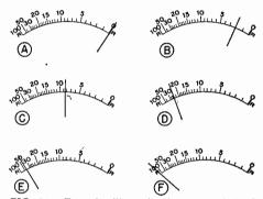
FIG. 21. Examples illustrating how to read the R scale on the meter of your N.R.I. Tester. The readings are as follows: A-0; B-2.0; C-8.5; D-24; E-40; F-1NFINITY.
