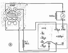
FIG. 25. Schematic (A) and semi-pictorial (B) diagrams for the triode vacuum tube circuit which you set up for Experiment 19.
