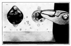
FIG. 6. This illustration shows the correct position of the bakelite mounting piece on the chassis, with the electrolytic condenser in position, and also shows how the outer lugs of the condenser are twisted a small amount with pliers to fasten the condenser unit to the bakelite mounting piece. Two of the lugs have already been twisted, and the last one is being twisted in this illustration.
