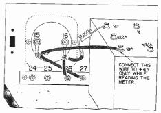
FIG. 19. Rear view of panel, showing connections for the shunt ohmmeter which you set up in Step 2 of Experiment 16.
