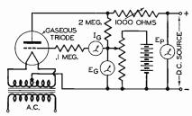
FIG. 20. Characteristic curves of a typical hotcathode gas filled tube, the Westinghouse type KU-610 grid-glow tube. D.C. starting characteristics for rated anode current are given at the left; the test circuit used appears above.
