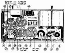
Fig. 3.—Bottom View of Chassis, Showing Parts
