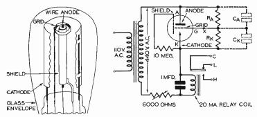
FIG. 22. Cut-away view of a cold-cathode grid-glow tube, showing arrangement of electrodes. The anode is inside a porcelain tube which in turn is surrounded by a metal cylinder, the shield. The grid is simply a thin band or ring of metal surrounding the exposed tip of the anode.
