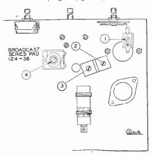
Figure 1. Bottom View Showing Trimmers
