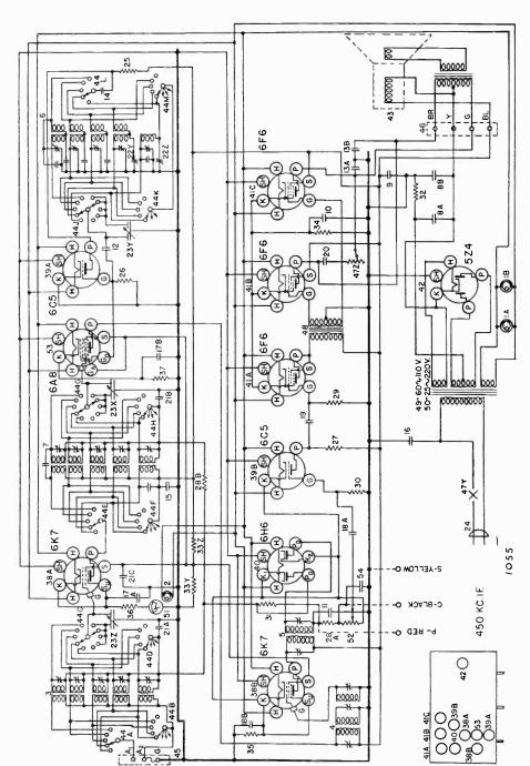
WIRING DIAGRAM—MODEL 1055
