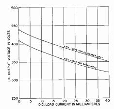
GRAPH 32DC. Plot your results for Experiment 32DC on this graph and draw a smooth line through the dots to secure a d.c. load current-d.c. output voltage curve for condenser input. Later, you will use values obtained in Experiment 34DC to plot another curve on this graph for a choke input type of filter circuit.
