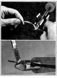
FIG. 17. Method of holding the solder and wire when tinning either solid or stranded wire. The heated soldering iron is left in its holder. The close-up photo shows a partly tinned wire. Slide the wire back and forth between the soldering iron tip and the solder until it is completely tinned for about half an inch from the end.
