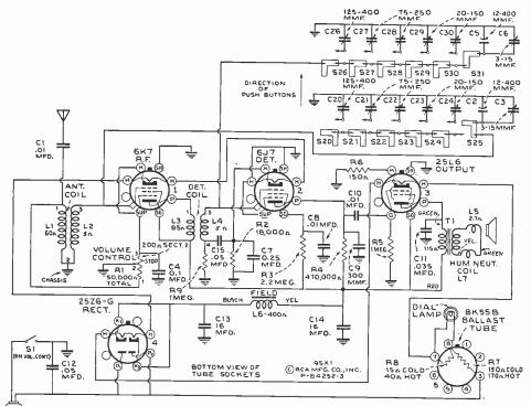
Schematic Circuit Diagram. The line by-pass, C12, is changed to .25 mfd. (Stock No. 12484) in some sets.
