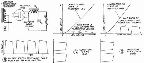
FIG. 25. These diagrams and the corresponding discussion in Experiment 35DC explain why the a.c. filter input voltage is higher for full load than for no load when your d.c. power pack is connected for choke input and full-wave rectification.
