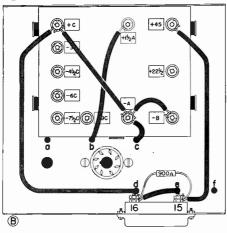
FIG. 24. Connections under the chassis for Step 2 in Experiment 18 should be as shown at A. The changes involved are as follows: Remove the lead which connects terminals 5 and 7, then bring a lead through hole d and connect it to terminal 5. Connections above the chassis should be changed to those shown at B. You now use the C terminals on the battery block for the first time.
