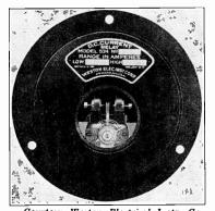
Courtesy Weston Electrical Instr. Co. FIG. 1B. Weston Model 534 meter type relay, capable of operating on coil currents as low as 15 microamperes.
