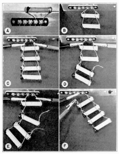
FIG. 20. Methods of connecting resistors to the d.c. output terminals of your power pack for d.c. output voltage and d.c. load current measurements are illustrated here. In all cases, there should be an external ground wire going to terminal group 2-5-4 as a safety precaution while the power pack is in see. Note that current is measured at the grounded point (\*terminal 4) in the load circuit; this keeps the chassis of the N.R.I. Tester at ground potential.
