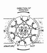
Fig. 10B. Cross-section view of simple two-pole d.c. generator, looking from the end opposite the commutator. A and B are brushes, while a, b, c, d, e and f are commutator segments.
