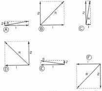
Fig. 24. The magnetic fields produced by coils at right angles to each other are shown as I and 2. Since the coils are fed 90° out of phase, I will be a maximum when 2 is zero, and vice versa. Since each field varies cyclically we have the conditions shown in A to F. If the net field is determined by addition, taking phase into account, we get the resultant R, which revolves at constant strength and therefore represents a revolving field.
