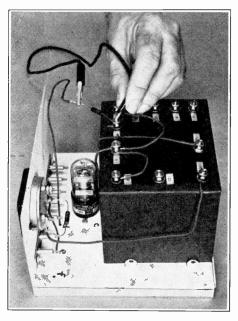
FIG. 27. Method of using a test lead to short out temporarily the grid resistor employed in Experiment 19.
