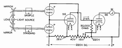
FIG. 19. Typical light differential circuit. The power supply is not shown, but should produce 220 volts D.C.; two separate 2.5 volt secondary windings are needed for XX and YY to prevent leakage reaction between the two amplifier tubes.
