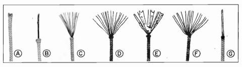
FIG. 18. Steps in preparing one end of the No. 18 stranded untinned lamp cord (Part 1-7G) which has rubber insulation covered with cotton braid. A—Original wire; B—wire with insulation removed from end; C—Strands spread out for cleaning; D—Cleaned strands ready to be tinned; E—Completely tinned strands; F—Tinned strands after surplus solder has been removed; G—Tinned strands twisted together again.
