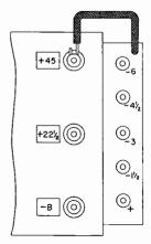
FIG. 47. Method of connecting an extra 7½-volt C battery to the B battery terminal of the special A-B-C battery block (or to the B battery itself if individual batteries are used) in order to compensate for a low B battery voltage.
