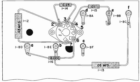
FIG. 38. The five radio parts which you connect to lugs in Experiment 9 are shown here ready for soldering. If you prefer, you can prepare all the parts in this manner, and then solder all the joints at once instead of soldering each part separately as called for in the experiment. WARNING: Bends in resistor and condenser leads should be gradual (not sharp), and should begin at least one-quarter inch away from the body of the part; otherwise, the leads will break off.
