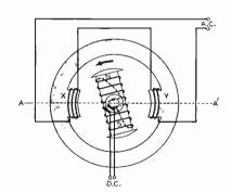
Fig. 21. A simplified a.c. synchronous motor.
