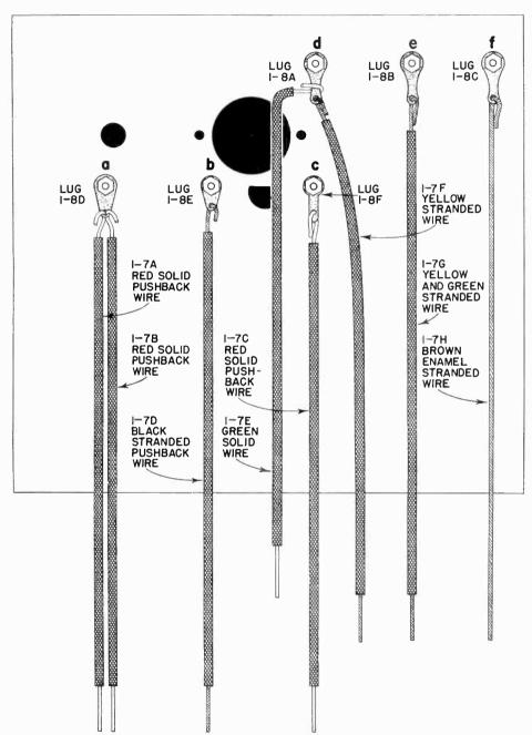
FIG. 27. Appearance of bottom of chassis after completion of Experiment 6. Each of the soldering lug connections commonly used by radio men is included in this experiment.
