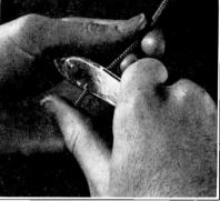
FIG. 13. When the insulation on a wire is too tough to be broken by squeezing with pliers, the pocket knife technique illustrated here is employed by some radio men for cutting through the outer braided covering on the wire. The knife must be sharp, and must be held lightly so as to avoid cutting too far and nicking or breaking the copper wire.
