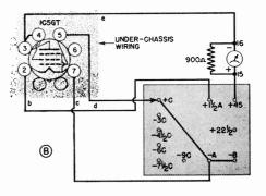
Insert the tube in its socket, read the meter on scale  $I_{\rm M}$  for this condition whereby the plate voltage is 45 volts and the control grid voltage is 0 volts with respect to the cathode. and record your results (first the meter reading, then the actual current in ma.) on the third line in Table 18.
