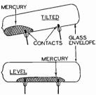
FIG. 11A (above). Tilted and level positions of a simple mercury switch, where a globule of mercury makes electrical connection between the two contacts.
