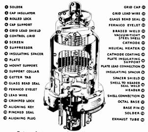
Internal structure of an all-metal radio tube.
