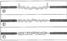
FIG. 29. Steps in connecting two wires together permanently by means of a Western Union soldered splice.
