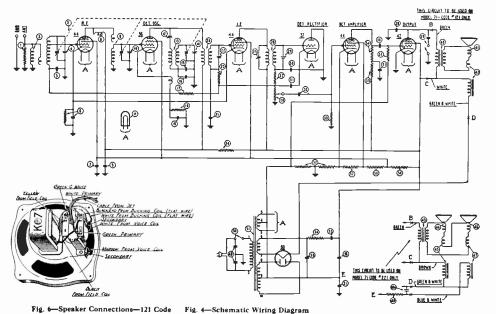
Fig. 4—Schematic Wiring Diagram DET OSCILLATOR 0 (26) (31) DET. AMPLIFIER DUTPUT DET RECTIFIER SOCKET SOCKET \$0EKET
