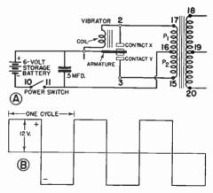
Fig. 11. Schematic circuit diagram (A) of the vibrator circuit in your d.c. power pack, and wave form (B) of the a.c. voltage which is applied to terminals 15 and 17 of the vibrator transformer primary winding by the vibrator.
