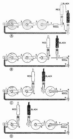
FIG. 12. Use these four milliammeter connections to prove for yourself that the same current value flows through all points in a series circuit.
