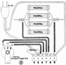
FIG. 25. Schematic (A) and semi-pictorial (B) circuit diagrams for the a.c. power supply source which you set up in Step 1 of Experiment 28.
