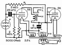
FIG. 17B. Another form of impulse circuit, which uses an extra tube to secure D.C. Here the relay pulls up only when light on the cell is suddenly interrupted, and drops out automatically in a definite time interval. Current flows through the tube circuits only during the half of each cycle for which polarity is as indicated.
