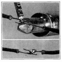
FIG. 28A (above). Correct way to solder a temporary hook joint. The tip of the iron is held under the joint, and the solder is applied to the wire from above.
