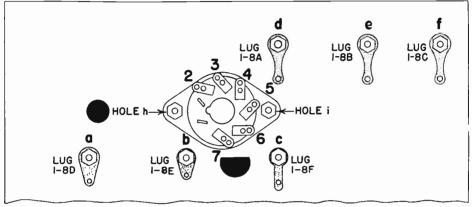
FIG. 37. Your chassis should appear exactly like this after you complete Step 1 in Experiment 9.
