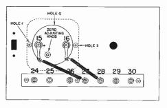
FIG. 6. Rear view of front panel, showing how the meter and jack strip are mounted and connected together for the experiments which are to be made before assembling the N. R. I. Tester. The chassis is not shown in this view, but should be attached to the bottom of the panel according to instructions given in Step 2 of Experiment 11.
