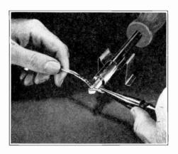
FIG. 22. Method of tinning a lug prior to mounting it on a chassis. This technique is used only for untinned lugs, or for tinned lugs which have become coated with oxides and dirt.
