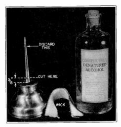
FIG. 5. Parts needed for making an alcohol lamp which can be used for heating a plain soldering iron, for removing enamel from wires, and for heating an electric soldering iron in locations where power is not available.
