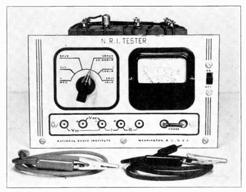
FIG. 33. Your N. R. I. Tester should look like this after you have assembled it according to the simple step-by-step instructions in this manual. The battery wiring will be modified, as explained later, if you use individual batteries in place of the special A.B.C battery block shown here.
