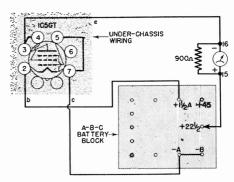
FIG. 22. Semi-pictorial wiring diagram for Step 1 of Experiment 18, in which you change the plate voltage on a diode tube from 22½ volts to 45 volts and note the effect upon plate current. The lead going to +22½ on the battery block is marked with an arrow to indicate that it is moved during the experiment.
