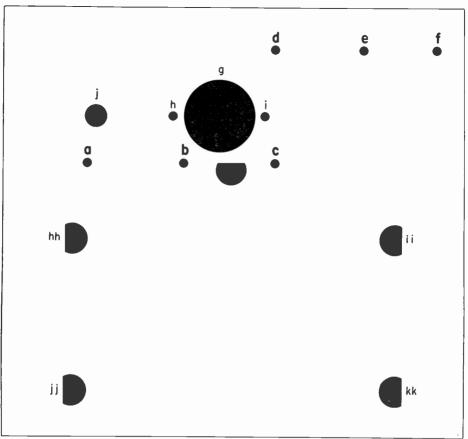
FIG. 19. Bottom view of metal chassis (supplied to you with Radio Kit 1RK, as Part 1-11). The front edge of the chassis has three holes and is bent in the same direction as the sides. The back edge of the chassis has no holes, and is bent in the opposite direction from the other three edges. The large letters a, b, c, d, e and f can be placed alongside the holes with a metal-marking crayon, ordinary soft lead pencil, or with pen and ink.
