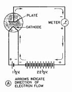
FIG. 20. Schematic circuit diagram (A) and semi-pictorial wiring diagram (B) for Step I of Experiment 17, in which you connect your type 1C5GT tube as a diode. The shaded area around the tube symbol in B indicates that connections to the tube socket are under the chassis. The letters e, b and c around this shaded area indicate the chassis holes through which the leads are run.
