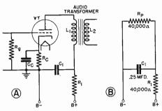
FIG. 29. Schematic circuit diagram of a typical vacuum tube stage (A), and equivalent circuit diagram for this vacuum tube stage as used in Experiment 39DC.
