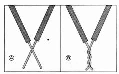
FIG. 30. Steps in making a common twist splice. This permanent joint is also known as a Bell splice, since it is used extensively by Bell Telephone linemen and switchboard men for connecting telephone wires together. When making this joint with solid wire, remove insulation for about 1 1/2 inches from the end of each wire, twist up to about 1/4 inch from the ends, then cut off the surplus wire with your side-cutting pliers.
