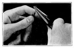
FIG. 24. Forming a hook on solid wire with long-nose pliers, preparatory to making a soldered hook joint.
