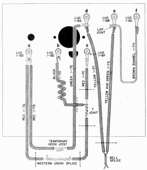
FIG. 34. Your chassis should appear like this after you have completed each of the joints called for in this experiment. The dotted lines indicate the approximate positions at which cuts should be made after completing this experiment so you can remove and save the T joint and the two splices,
