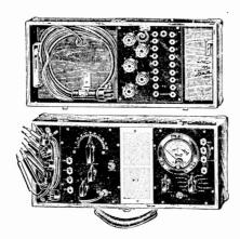
Tool or aid for Servicemen. This tester consists of an all-wave signal generator, a multimeter and a plug-in system. Your course will show and explain how these service tools are used.
