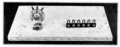
FIG. 12. For Step 1 of Experiment 28DC, mount the terminal strip and the potentiometer bracket in approximately the positions shown here, on a wood baseboard approximately ½-inch thick, 5 inches wide and 7 inches long.
