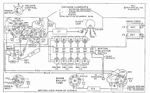
RADIOTRON SOCKET VOLTAGES, AND LOCATION OF PARTS
