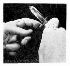
FIG. 12. Always use the portion of your pocket knife blade closest to the handle for scraping oxides and dirt from exposed copper wire preparatory to soldering. This preserves the main part of the blade for purposes where sharpness is required, such as when cutting through braided cotton insulation.
