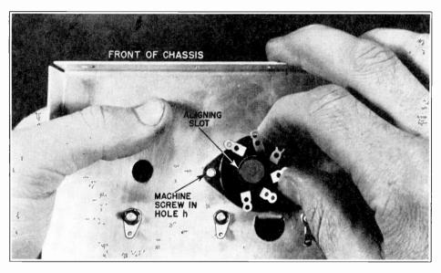
FIG. 36. Method of mounting the tube socket on the chassis. The terminal lugs of the socket should be underneath the chassis, and the aligning slot should be at the left (near hole h) when the chassis is held as shown in this illustration. Hold the machine screw in position with a finger of your left hand.
