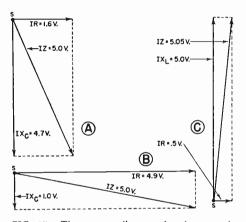
FIG. 17. These vector diagrams, based upon voltage values measured in the N.R.I. laboratory for the various steps in Experiment 28DC, prove definitely that Kirchhoff's Voltage Law holds true for a.c. circuits.
