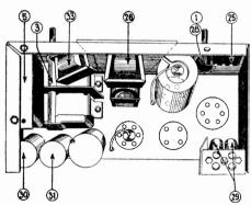
Fig. 2-Top View of Chassis, Showing Parts
