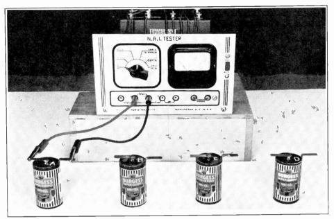
FIG. 3. Method of using the N.R.I. Tester to measure the voltages of individual dry cells. This set-up is used in Step 3 of Experiment 21. The test leads were shortened for this photograph in order to make them show more clearly, but do not shorten your own test leads. Placing the N.R.I. Tester on a box makes it easier to read the meter accurately.
