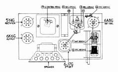
Fig. 1. Location of Compensators
