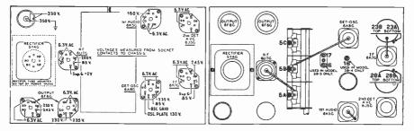
Socket Voltages-Underside of Chassis View
