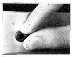
FIG. 4. Squeeze the grommet for the power line cord between your thumb and forefinger in the manner shown here while forcing it into hole u in the side of the chassis. This grommet can be placed in position with your fingers; it may take a little time at first, but you will soon get the "knack" of doing this radio job.
