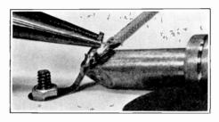
FIG. 35. Method of unsoldering a permanent hook joint on a soldered lug. Spread open the hook with long-nose pliers while keeping the solder molten by holding the soldering iron under the lug.
