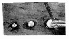
FIG. 9. Method of increasing the size of a molten globule of solder by feeding rosin-core solder to the soldering iron tip while it is in contact with the globule. The three globules used in Experiment 2 are shown clearly in this view. The darker rings on the board around each globule are formed by the surplus rosin flux, which is a yellowish liquid when heated.
