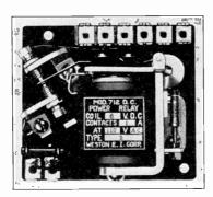
Courtesy Weston Electrical Instr. Co. FIG. 4A. Weston Model 712 D.C. sensitive relay, capable of handling up to 1 ampere at 110 volts A.C. The coil is wound for 6 volts D.C. The common contacts are here mounted on a thin springy blade attached to the armature; this gives a wiping motion at the contacts, which tends to keep them Clean.
