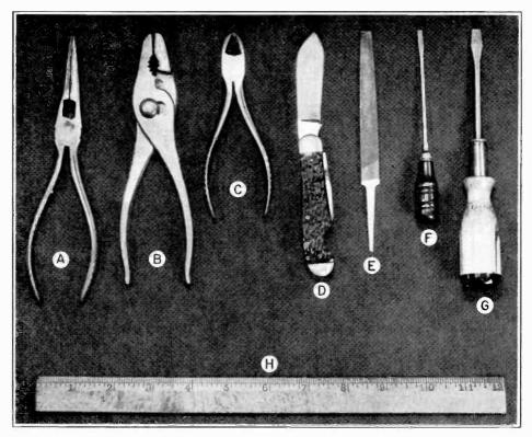
FIG. 2. The essential tools which you will need for the experiments in your practical demonstration course are pictured here and identified below. Get the best side-cutting pliers and long-nose pliers you can afford, for you will use these tools continually throughout your practical demonstration course and in actual radio work of all kinds.
