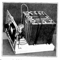
FIG. 44. The diagram at the left is a partial rear view of the completed N.R.I. Tester, showing how the length of black lace (Part 2-20) can be used to tie down the special Burgess A.B.C battery block. The photograph shows how the battery block actually appears after wiring is completed and the lace put on; an optional position for the lace between tabs ii and jj is shown in this photo.
