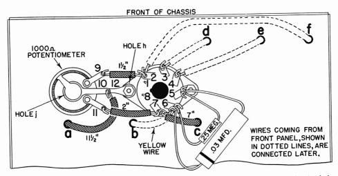
FIG. 41. Bottom view of chassis, showing preliminary assembly of leads and wires. After the chassis is bolted to the panel, four wires from the panel will be run through holes b, d, e and f and connected to terminals 6, 3, 4 and 2 respectively, as indicated by the dotted lines.
