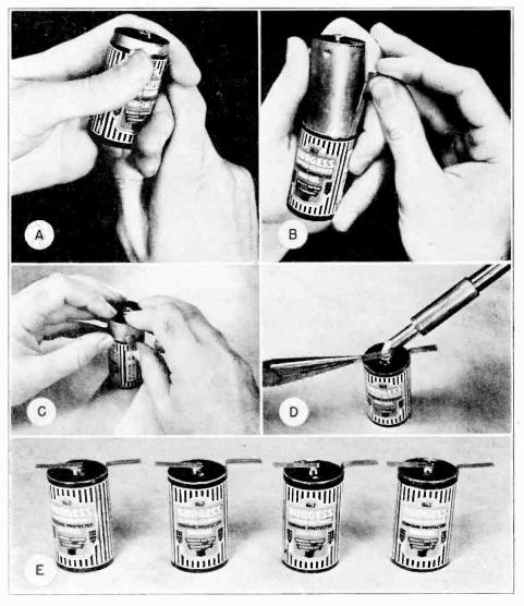
FIG. 4. Steps in providing the four 11/2-volt flashlight cells with convenient soldering terminals.
