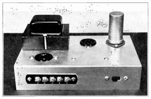
FIG. 7. Top view of the completed d.c. power pack chassis before the vibrator and rectifier tube have been inserted in their sockets.
