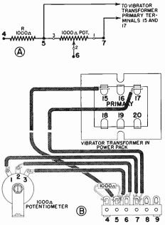
FIG. 13. Schematic (A) and semi-pictorial (B) circuit diagrams for the a.c. voltage divider which you set up according to the instructions given in Step 1 of Experiment 28DC.
