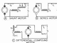
Fig. 16. Electrical circuits for three types of d.c. motors.
