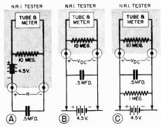
FIG. 16. Schematic circuit diagrams for Experiment 26.
