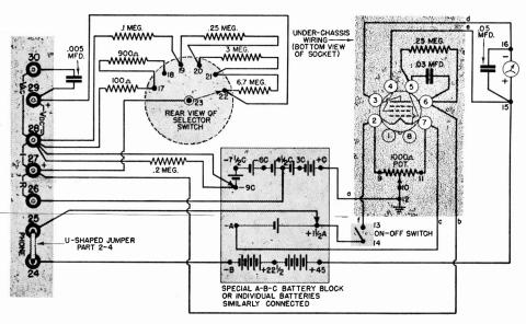
FIG. 34. Circuit diagram of the N. R. I. Tester. This is presented here for reference and checking purposes; you will follow pictorial diagrams and photographs when assembling the unit, to minimize chances for errors.
