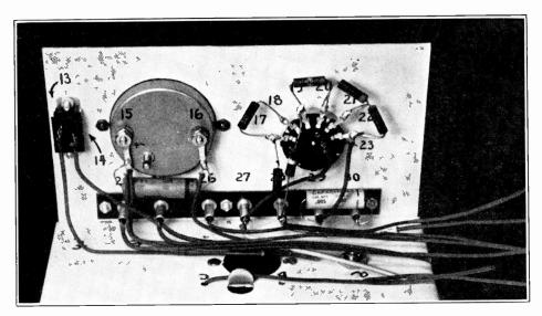
FIG. 42. Rear view of N. R. I. Tester after the panel is fastened to the chassis. Note that the leads have been temporarily bent off the chassis to the right to permit placing the battery block on the chassis between the five tabs. The position of the OUTSIDE FOIL lead of the condenser connected between meter terminals 15 and 16 does not matter, since neither meter terminal is grounded.
