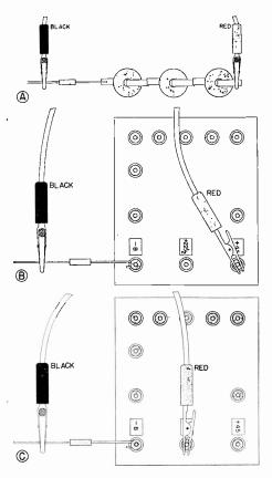
FIG. 13. The three circuits illustrated here all have the same total resistance (the meter with its resistance of 2,000 ohms is not shown, but is connected to the other ends of the two test leads in each case), but each circuit has a different voltage. In Experiment 14 you measure the current in each circuit and note its relationship to the circuit voltage, thereby demonstrating how a milliammeter can be used as a voltmeter.
