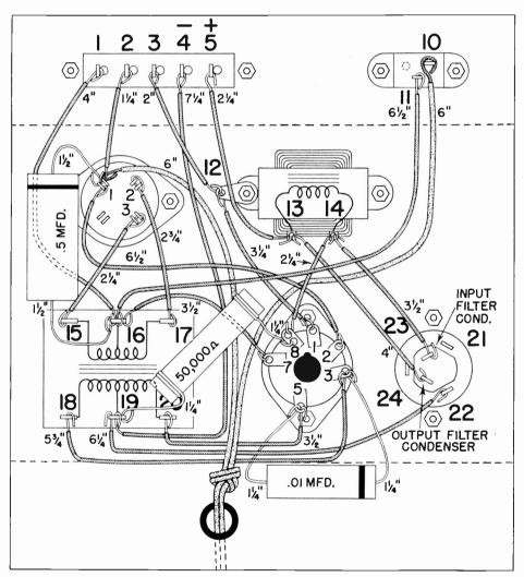
FIG. 8. Semi-pictorial wiring diagram showing how all connections are made under the chassis of the d.c. power pack. The sides of the chassis have been flattened out for clearness, but the wire lengths specified on this diagram are correct for the actual chassis.
