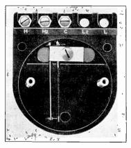
Courtesy Weston Electrical Instr. Co. FIG. 12B. Weston Model 613 time delay relay with cover removed. Heater coil requires 6 volts D.C., while contacts will control 25 watts.
