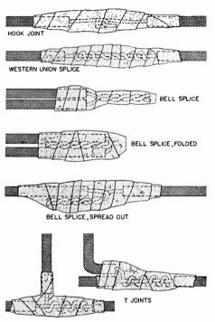
FIG. 33. Methods of taping the various types of soldered joints taken up in this manual. These diagrams are presented for future reference only, since you do not have to tape any of the joints used in your practical demonstration course.
