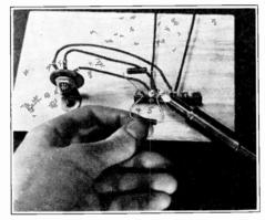
FIG. 16. This illustration shows you how to make a temporary soldered lap joint for the purpose of connecting a radio part such as a resistor temporarily between two terminals. If the parts being connected together are liberally tinned beforehand, this technique allows you to hold the part with one hand (instead of holding solder in that hand), and gives a joint which can easily be disconnected.
