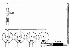
FIG. 8. Cell connections and test clip positions for Step 8 of Experiment 21.
