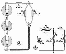
FIG. 12. Semi-pictorial and schematic circuit diagrams for Experiment 23.
