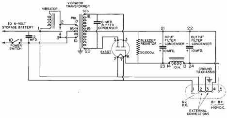
FIG. 2. Schematic circuit diagram for the d.c. power pack which you build before beginning the experiments in this manual. The terminals on this schematic diagram are numbered to correspond with the terminals shown on the semi-pictorial diagrams in Figs. 5 and 8.
