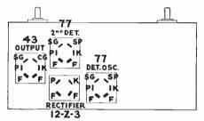
F Filament P Plate SG Screen Grid CG Control Grid K Cathode SP Suppressor Grid
