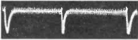
FIG. 26. Trace representing the output of the vertical integrating network.
