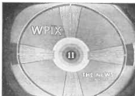
FIG. 24A. Light ignition interference causes streaks of this kind across the picture.
