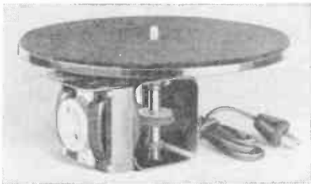
FIG. 40. A drive system that operates through the center spindle. This photo shows a record player; a changer would use a different spindle and would have the changer mechanism. These are omitted here to show the drive more clearly.
