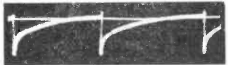
FIG. 27. Trace representing the wave shape at the grid of a vertical blocking oscillator.
