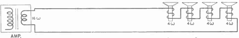
FIG. 14. Matching impedances of series-connected voice coils.
