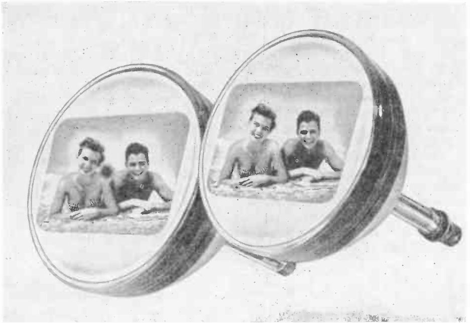
FIG. 26. Notice ion spot in center of the face of the tube at left.
