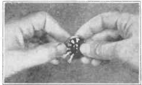
FIG. 35. Method of bending out the soldering lugs on the rotary selector switch (Part 2-6). Press them outward with your thumb, one at a time, until all the outer lugs point outward like the spokes of a wheel. Do not bend the single center lug.
