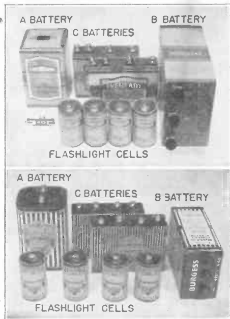
FIG. 3 The only batteries you need for Experiments 11 to 20 in this manual and for the NRI Tester are four standard No. 2 (large size) flashlight cells, one 1\frac{1}{2} -volt A battery, one 45-volt B battery and two 4\frac{1}{2} -volt C batteries. These can be the Eveready or Burgess units shown here and specified below, or any other makes having exactly the same dimensions and terminal arrangements.
