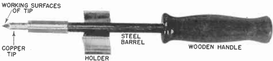
FIG. 6. This is called a plain soldering iron, as its working tip is heated in a flame. It is used where no electric power is available. A suitable heating device is described in the text.
