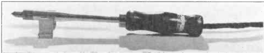
FIG. 4. This shows how to place your soldering iron on a metal holder. Note that the working tip is placed beyond the holder, so that it does not become cooler through contact with the metal which would carry off some of its heat.
