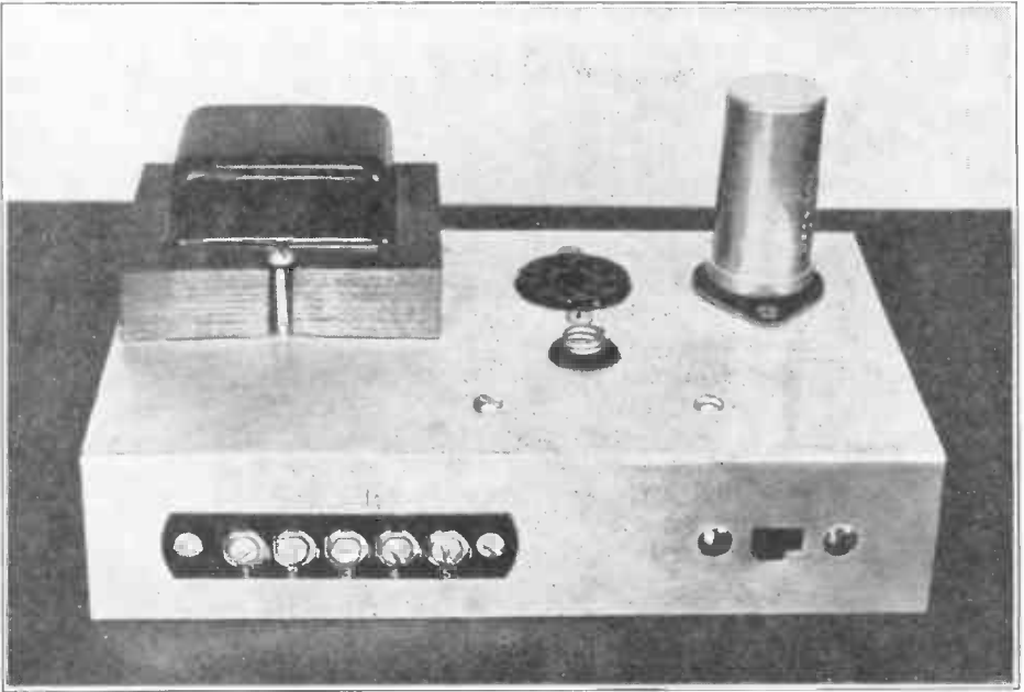
FIG. 7. View of the completed a.c. power pack before the rectifier tube and pilot lamp have been inserted in their sockets.
