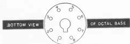
FIG. 34. The pin arrangement of an octal-based tube, which also corresponds to the bottom socket connections.
