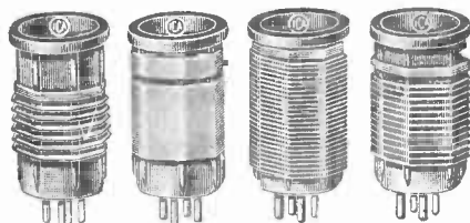
Examples of plug-in coils used in experimental short-wave receivers.
