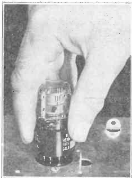
FIG. 21F. Hold a radio tube in the manner shown here when pushing it into or removing it from a socket. Make sure that the aligning key on the tube base is in the aligning slot on the tube socket before attempting to push a tube into its socket. Most of the downward pressure is applied by the thumb and forefinger gripping the base. It may be necessary to apply pressure also on the top of the glass envelope, and rock the tube gently from side to side while pushing downward, for the contacts in a new socket are sometimes a bit stiff. Use the same grip and rocking motion for pulling out the tube.
