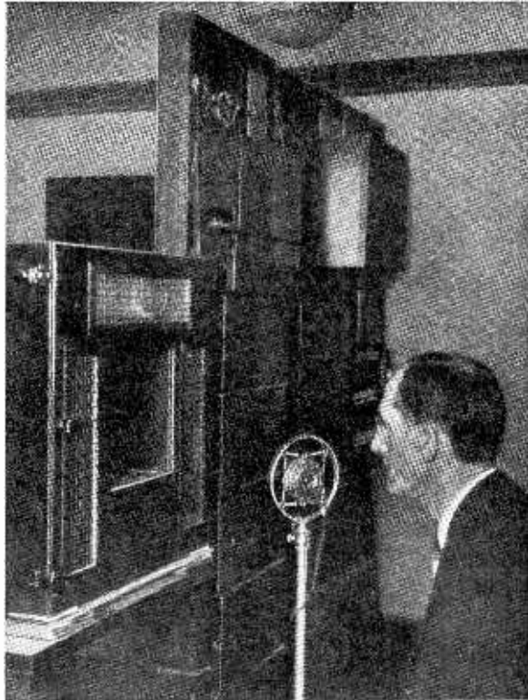
Fig. 3—A close-up of the transmitting apparatus for television at Washington, D. C. When a person talks to the microphone he is viewed by three photo-electric eyes located behind the three screens of the box immediately in front of him.
