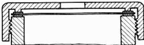
Fig. 16—Illustration showing how rubber gaskets are used in place of the rubber tubing, as shown in Figure 15.
