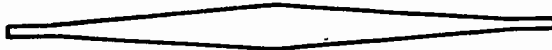
Fig. 14—A type of diaphragm made of a non-magnetic material, the thickness at the center being greater than at its edges.
