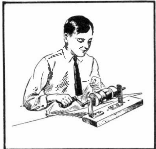
FIG. 1 SET-UP FOR WINDING R. F. TRANSFORMER
