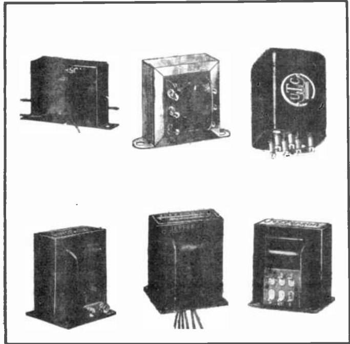
FIG. 10 TYPICAL A-F TRANSFORMERS
