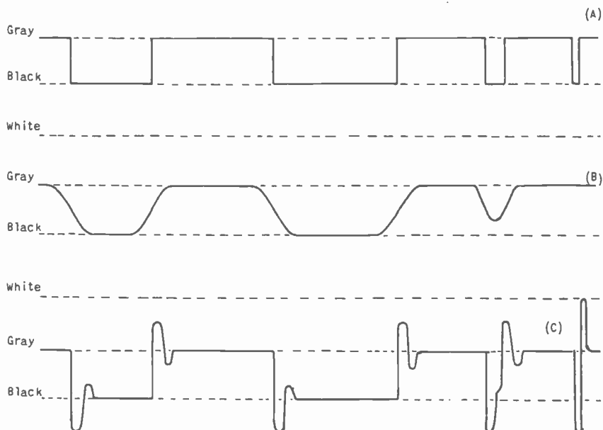
Fig. 14 (A) waveform generated in scanning vertical black bars on a gray background, (B) distortion of the waveform caused by low high-frequency gain, and (C) the distortion caused by excessive high-frequency gain.
