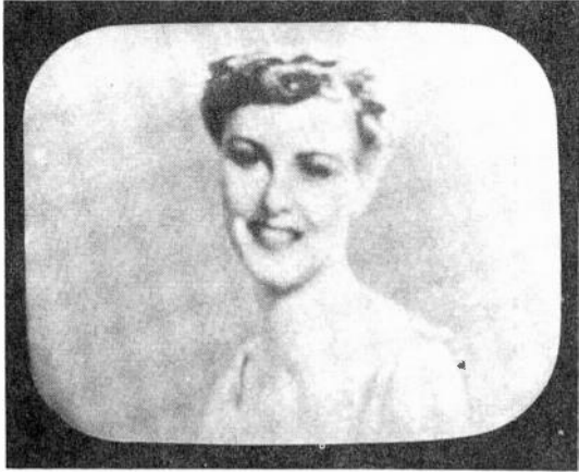
Fig.18 Incorrect vertical linearity.
