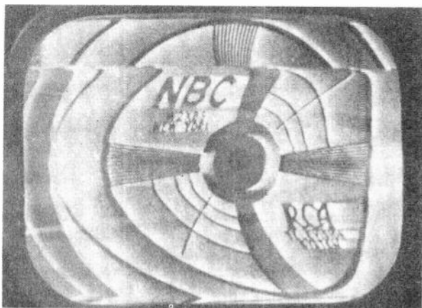
Fig. 11 Effect of excessive signal strength.
