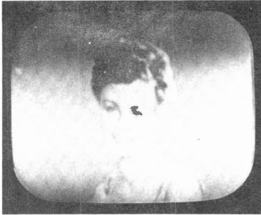
Fig.21 Sixty cycle hum in the video circuits.
