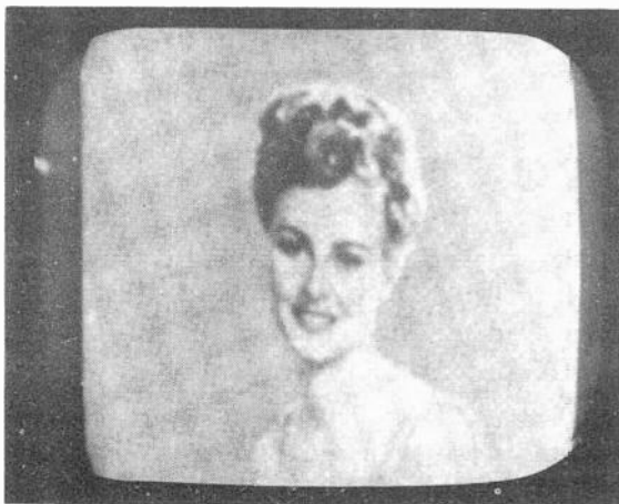
Fig.1 Insufficient horizontal deflection.
