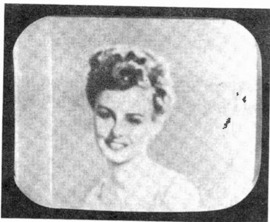
Fig. 31 Effect of horizontal damping tube failure.
