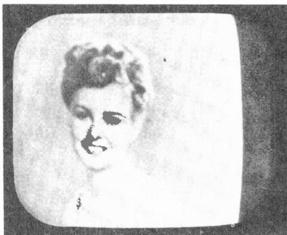
Fig.17 Misadjustment of horizontal centering control.
