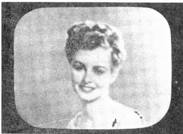
Fig. 15 Cross-hatching due to interference from a radio frequency carrier.
