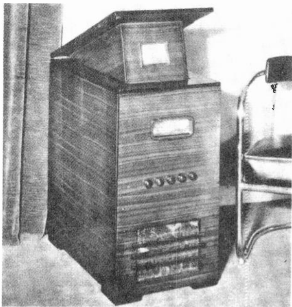
The Garod Model 100 television receiver, mounted in a console together with an all-wave sound receiver.
