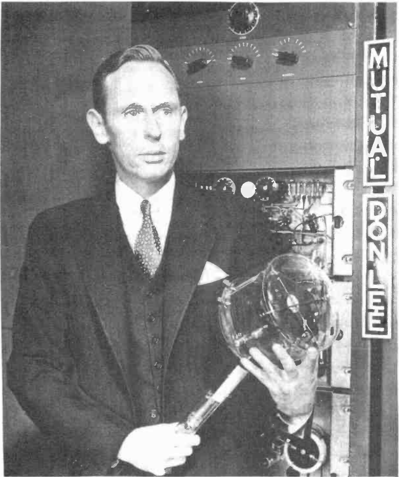
Fig.10 Mr. Lubke, Chief Engineer of W6XA0, shown with portion of the equipment at that station. He is holding late model iconoscope.
