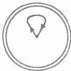
Fig. 14 Path of an electron in focusing coil when viewed along axis of coil.
