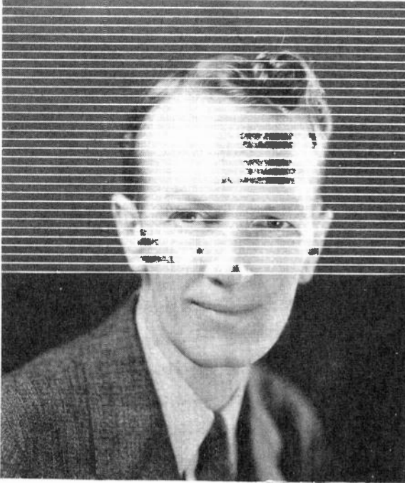
Fig.7 Showing how the photograph in Fig. 6 is broken up into scanning strips.
